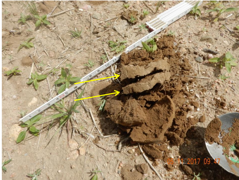
Photo 10: Photo shows a soil clod removed from the top 6-8 inches of the soil from the road. Photo shows “Platy” soil structures. Platy structures are thin, flat plates of soil that lie horizontally and are usually found in compacted soils. Yellow arrow seen points out some of the platy structures found.
