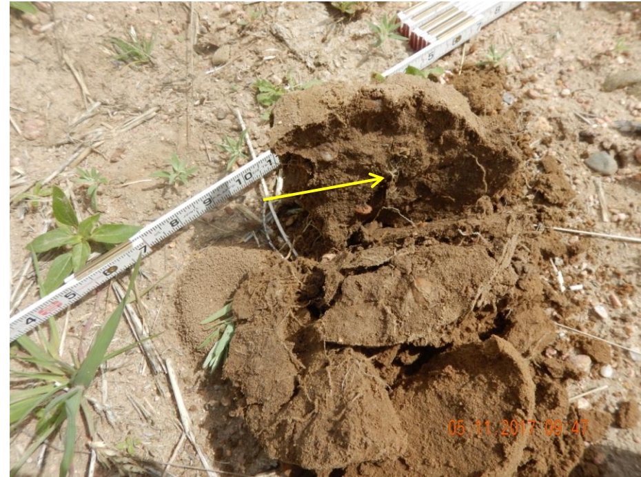
Photo 11: Photo shows a soil clod removed from the top 6-8 inches of the soil from the road. Photo shows “Platy” soil structures. Platy structures are thin, flat plates of soil that lie horizontally and are usually found in compacted soils. Arrow shows a layer of compaction that has hindered root penetration.
