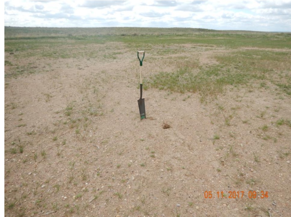
Photo 5: Photo taken from the location. Reclamation specialist tested location to see if compaction alleviation had been performed. Photo shows shovel was only able to penetrate soil ~2-3 inches before hitting a compaction zone.
