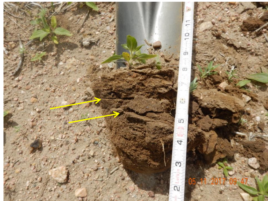
Photo 9: Photo shows a soil clod removed from the top 6-8 inches of the soil from the road. Photo shows "Platy" soil structures. Platy structures are thin, flat plates of soil that lie horizontally and are usually found in compacted soils. Yellow arrow seen points out some of the platy structures found.
