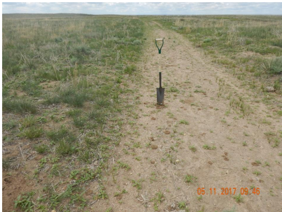
Photo 8: Photo taken from the location. Reclamation specialist tested location to see if compaction alleviation had been performed. Photo shows shovel was only able to penetrate soil ~2-3 inches before hitting a compaction zone.
