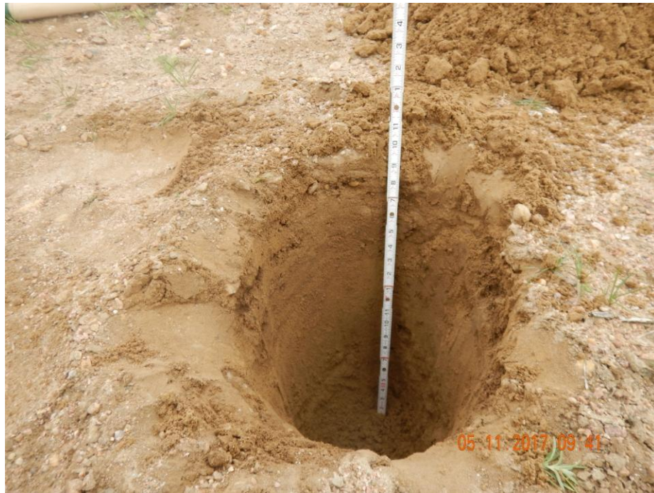
Photo 6: Photo taken from the location. Photo shows test pit dug by reclamation specialist to determine if compaction alleviation had been performed. Photo shows pit is ~20 inches deep.
