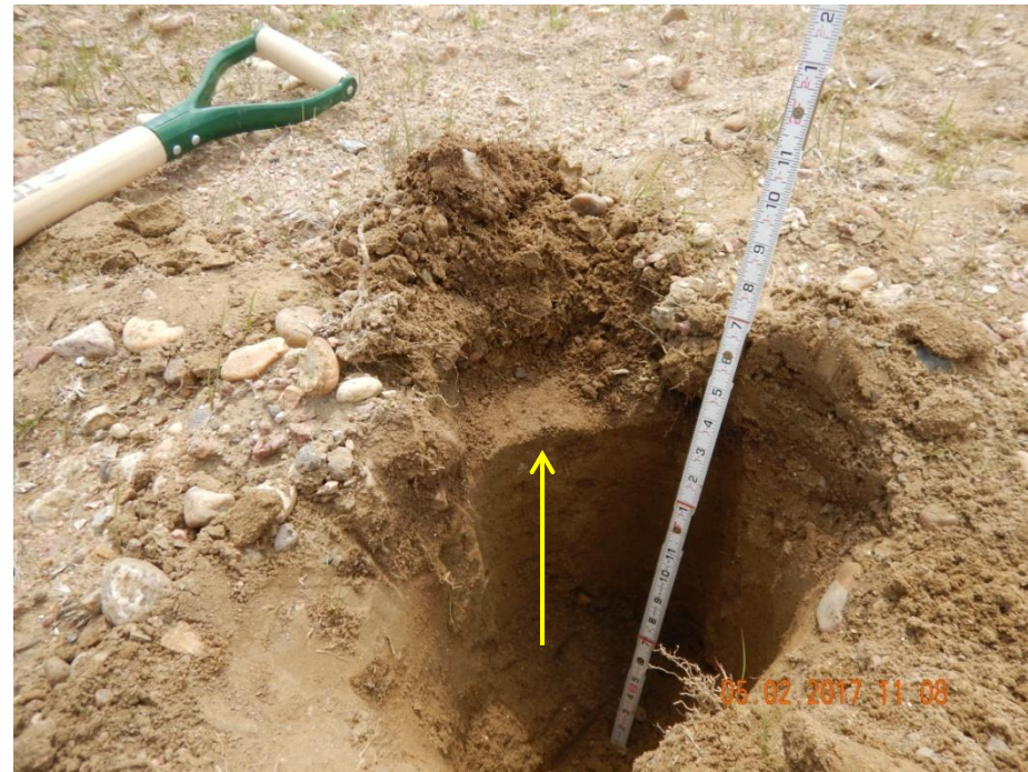
Photo 8: Photo shows test pit dug by reclamation specialist to determine if compaction alleviation had been performed. Photo shows a compaction zone beginning ~3-4 inches deep sub-surface (yellow arrow). The top 4 inches of soil was easily lifted off to reveal a "bench" at where compaction zone begins. Re-contour work may have been attempted followed by a seeding, however, this photo shows compaction alleviation had not been performed.
