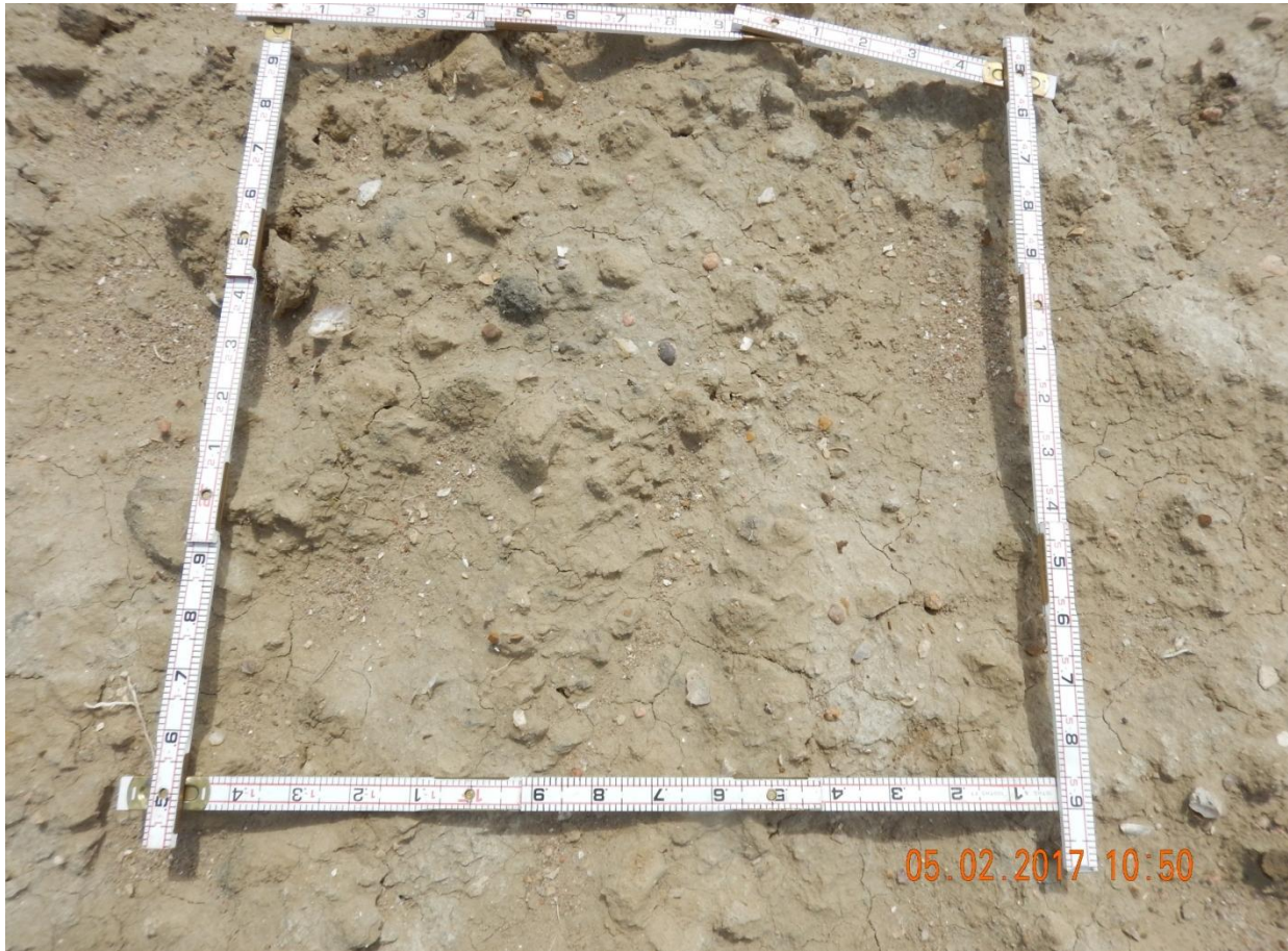
Photo 15: Photo taken from the southwest end of the location. Photo shows area of the location where vegetative germination is not evident. Continue to monitor this portion of the location and reseed if reclamation does not progress. . Quadrat is ~1.5 feet x 1.5 feet.
