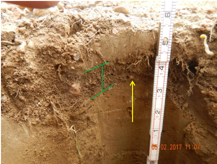
Photo 7: Photo shows test pit dug by reclamation specialist to determine if compaction alleviation had been performed. Photo shows a compaction zone beginning ~3-4 inches deep sub-surface (yellow arrow). Green line shows layer of subsoil where compaction has hindered water infiltration and root penetration by vegetation that had been previously established; very little organic matter (root development, etc...) was evident below area of compaction.
