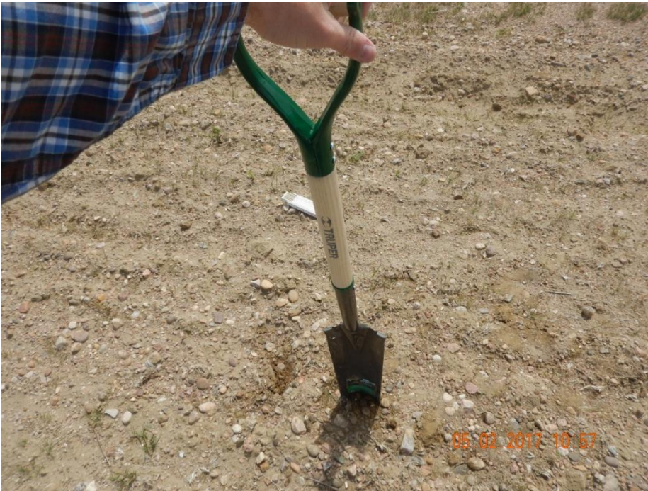
Photo 5: Photo taken from access road, west of the location. Reclamation specialist tested road to see if compaction alleviation had been performed. Photo shows shovel was only able to penetrate soil ~2-3 inches before hitting a compaction zone at ~3-4 inches.
