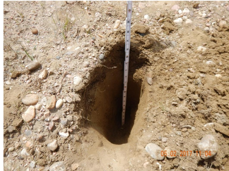
Photo 6: Photo taken from access road, west of the location. Photo shows test pit dug by reclamation specialist to determine if compaction alleviation had been performed. Photo shows pit is ~20 inches deep. A compaction zone had been identified beginning ~3-4 inches deep sub-surface.
