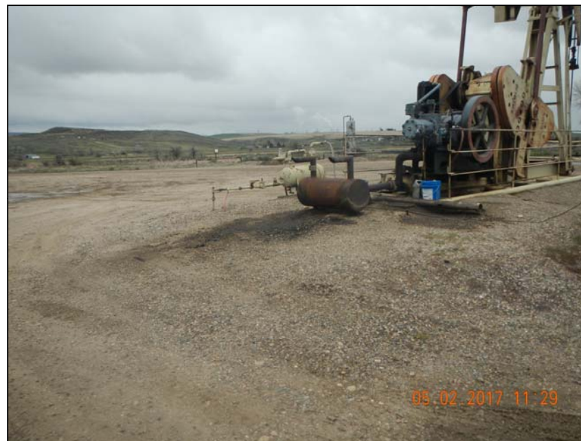
Photo 2. Stained soil at exhaust, lube oil containers without secondary containment.
