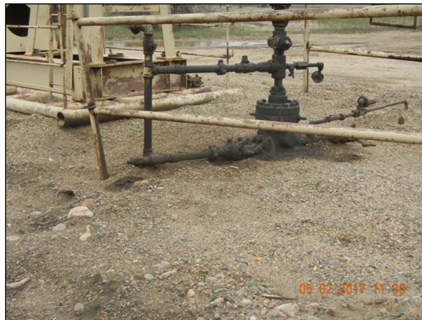
Photo 4. Stained soil at wellhead.
