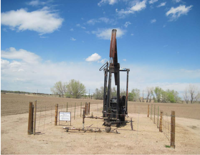
Wellhead and pump jack
