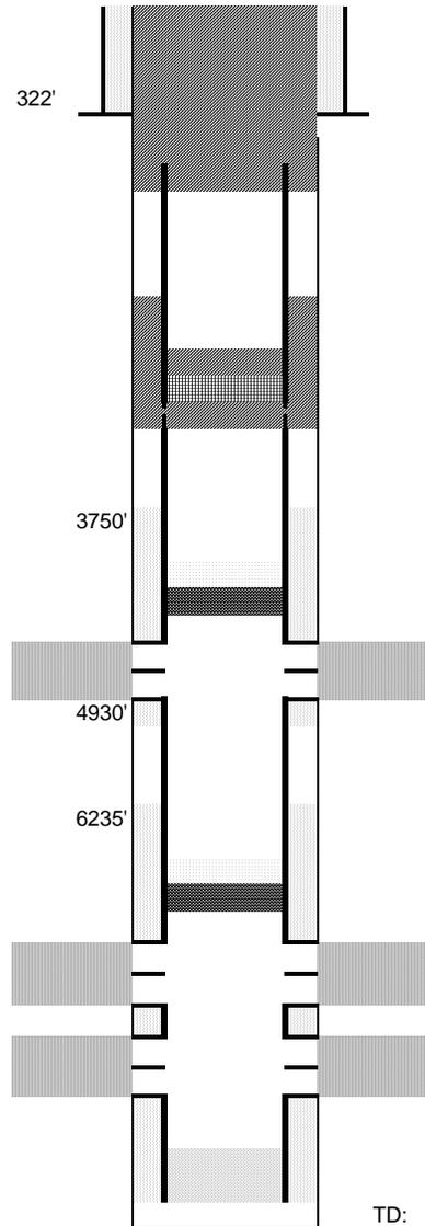
Cut surface casing off 6'-8' below surface.
