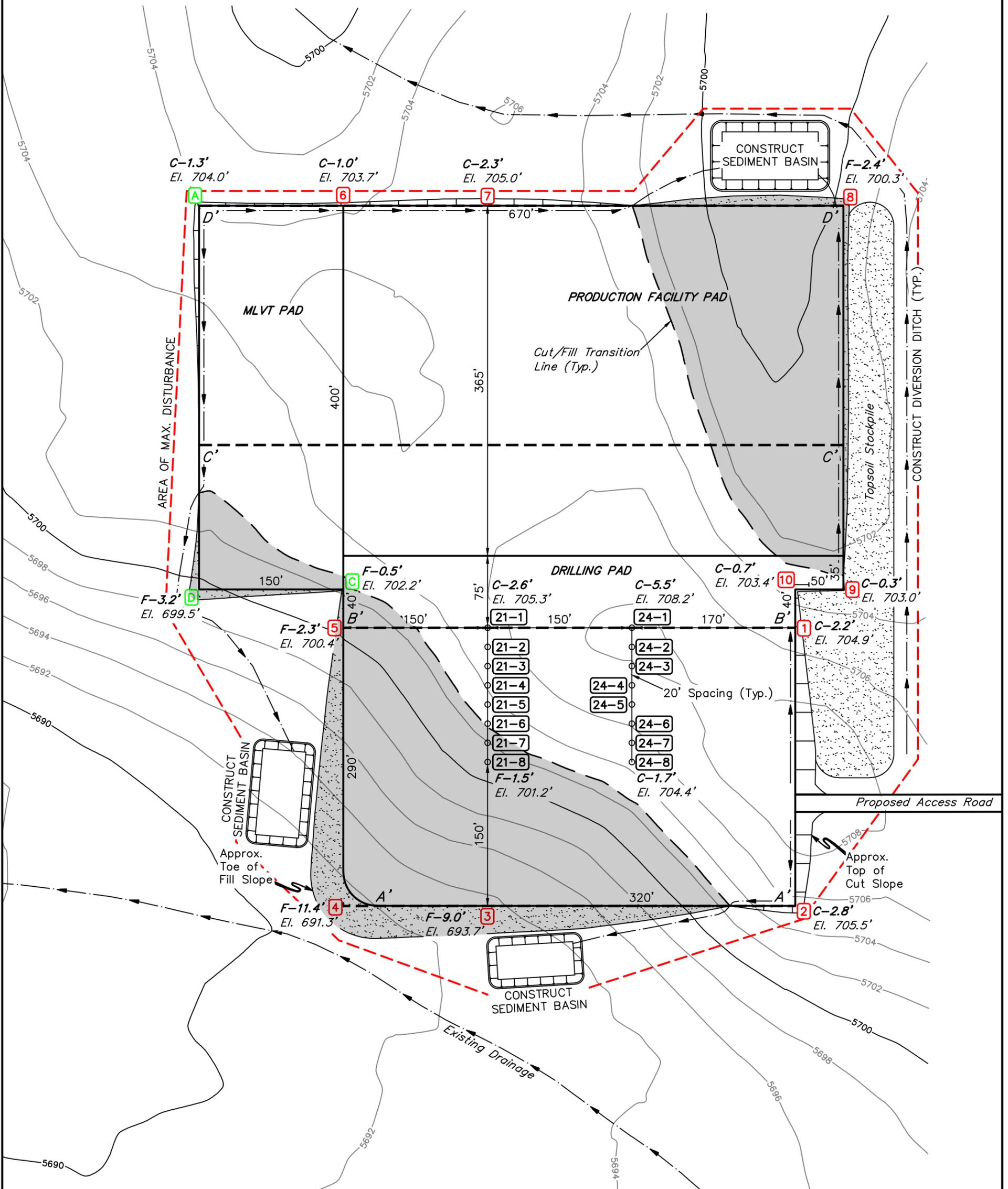
NOTE: Earthwork calculations require a fill @ some of the location stakes for balance. All fill is to be compacted to a minimum of 95% of the maximum dry density obtained by AASHTO method t-99.
