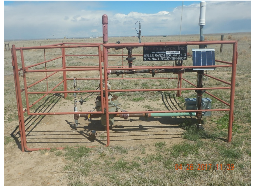
Photo 2: Wellhead, looking N
