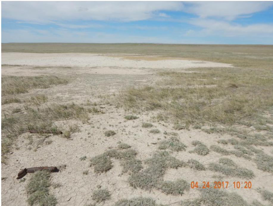
Photo 2: Photo taken from the northeast end of the location, facing southwest. Photo shows large areas of what appears to have been a salt kill that have not had any reclamation or stabilization performed. Photo also shows pipe debris remains on the location.
