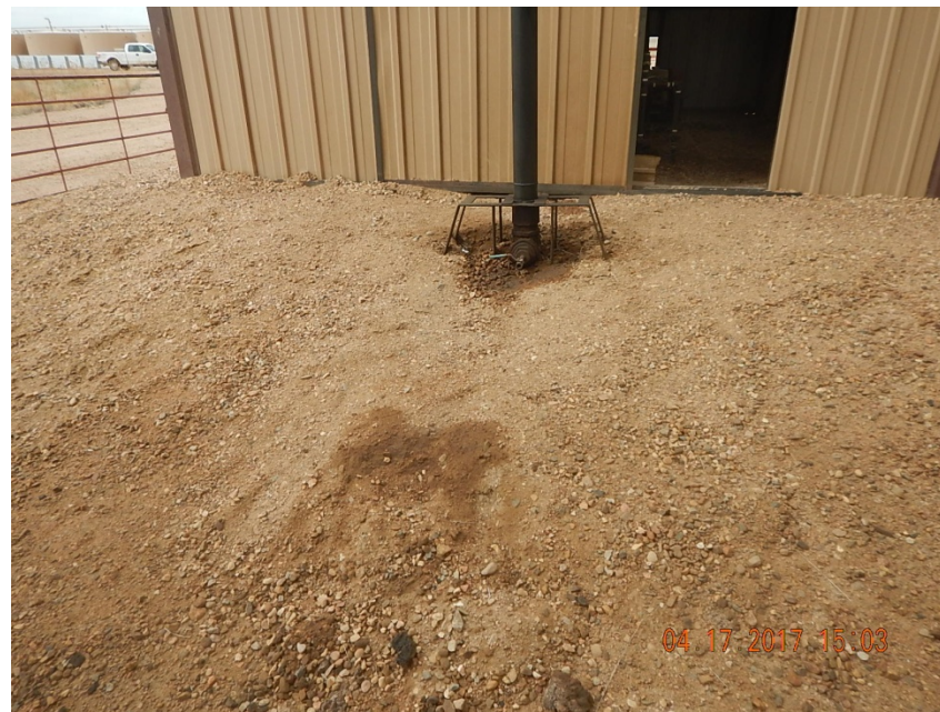
Photo 4: Stained soil at engine exhaust
