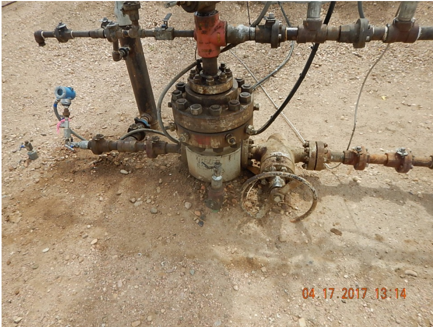
Photo 3: Stained soil at wellhead
