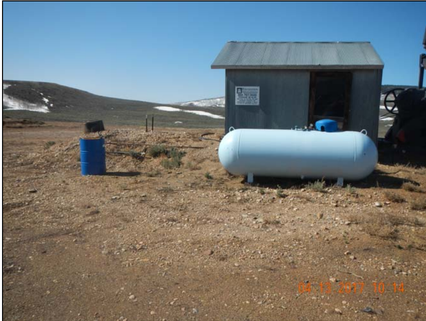
Photo 3. Unlabeled containers at wellhead. One without secondary containment.
