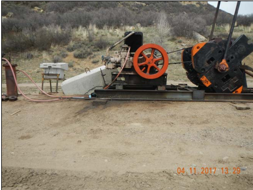
Photo 2. Stained soil at pump jack exhaust.
