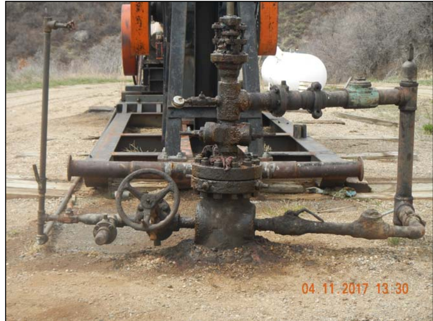
Photo 3. Stained soil at wellhead.
