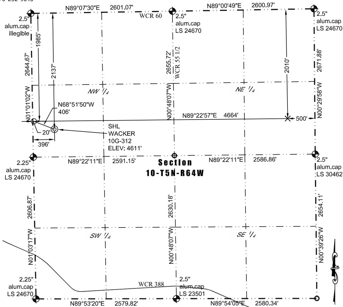
In accordance with a request from Mac Neumann of PDC Energy, Inc., Washburn Land Surveying, LLC has determined the location of the **WACKER 10G-312** well site to be SHL: 2137' FNL and 396' FWL, (BHL: 2010' FNL and 500' FEL), as measured at ninety (90) degrees from the section lines of Section 10, Township 5 North, Range 64 West of the 6th Principal Meridian, Weld County Colorado.
