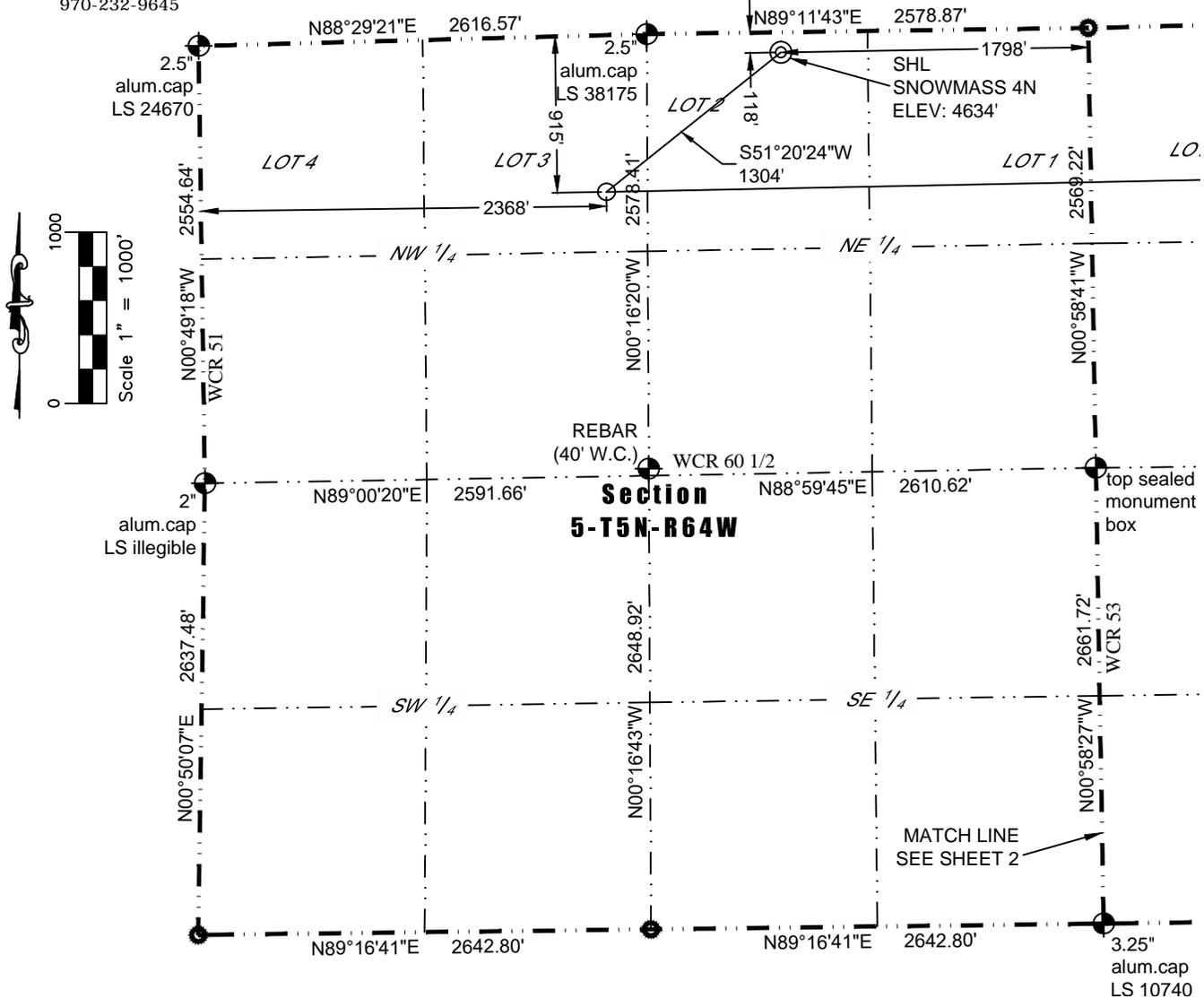
In accordance with a request from Paul Montville of PDC Energy, Inc., Washburn Land Surveying, LLC has determined the location of the **SNOWMASS 4N** well site to be SHL: 118' FNL and 1798' FEL, (BHL: 915' FNL and 0' FEL), as measured at ninety (90) degrees from the section lines of Sections 4 and 5, Township 5 North, Range 64 West of the 6th Principal Meridian, Weld County Colorado.
