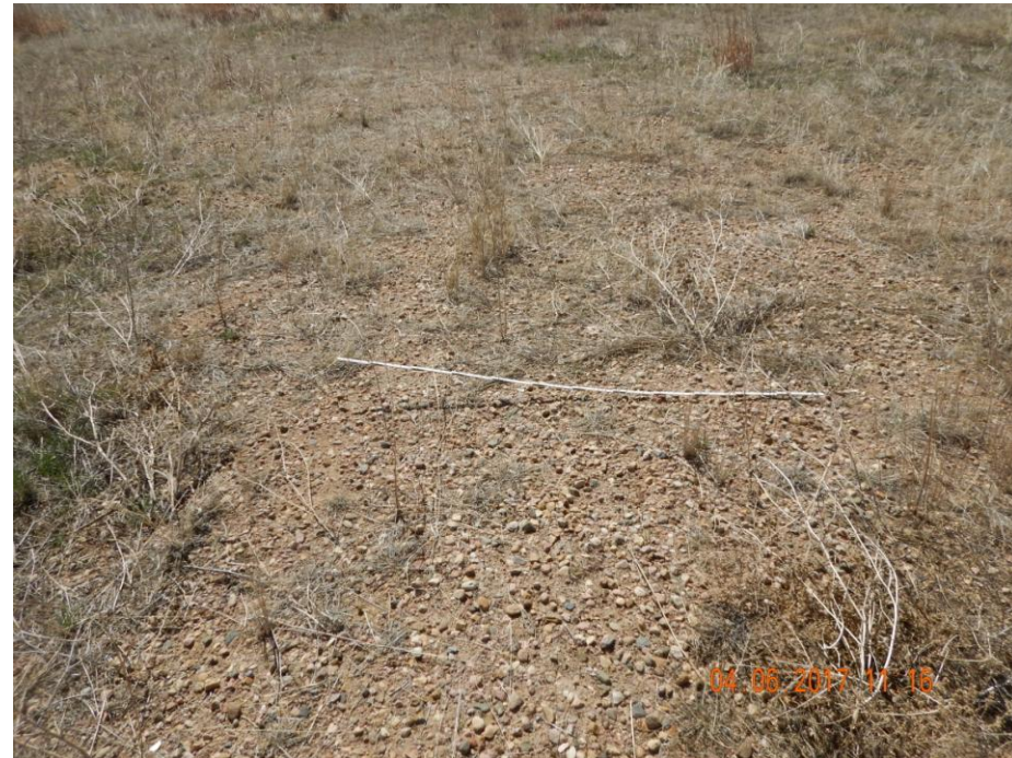
Photo 5: Photo taken from the location. Photo shows large portions of the location where gravel and base material have not been removed and remain unvegetated. 6 foot measuring stick for reference.
