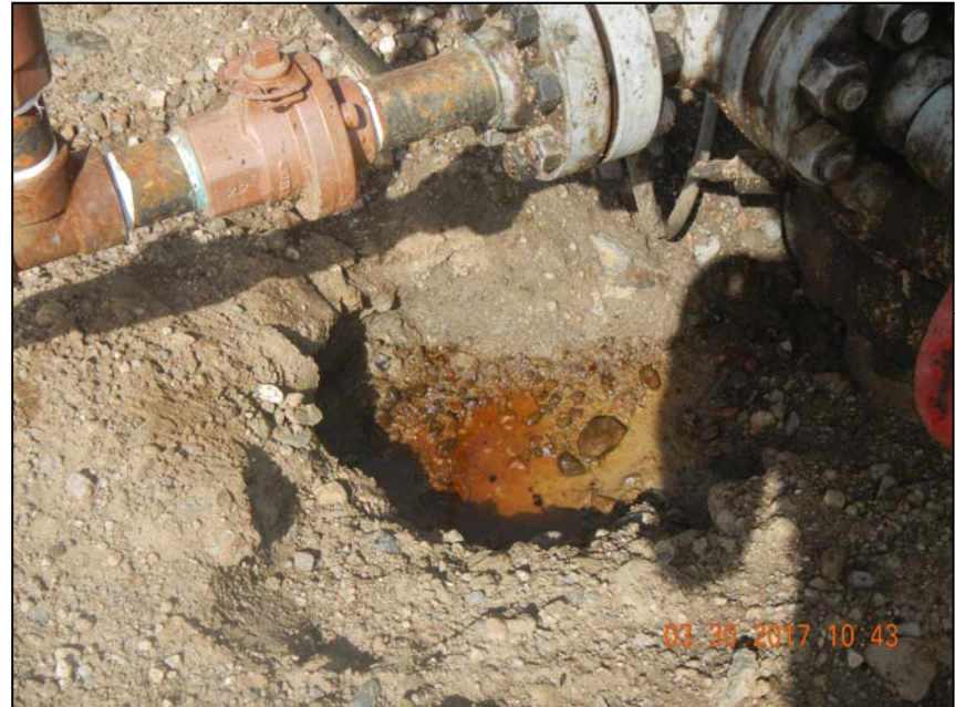
Photo 4. Subsidence with sheen on top of water.
