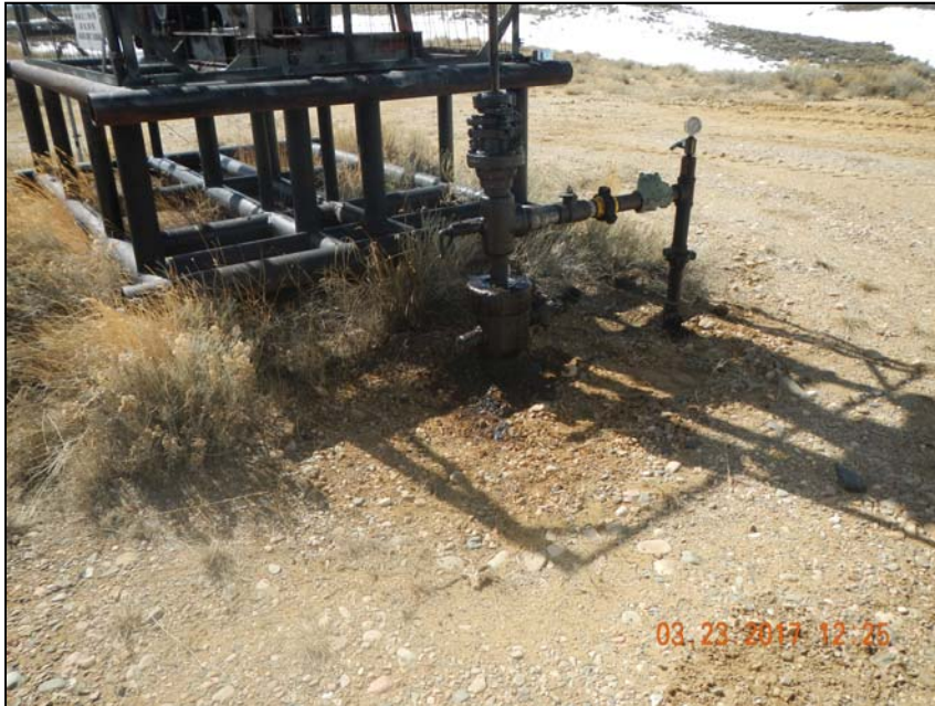
Photo 2. Stained soil at wellhead.
