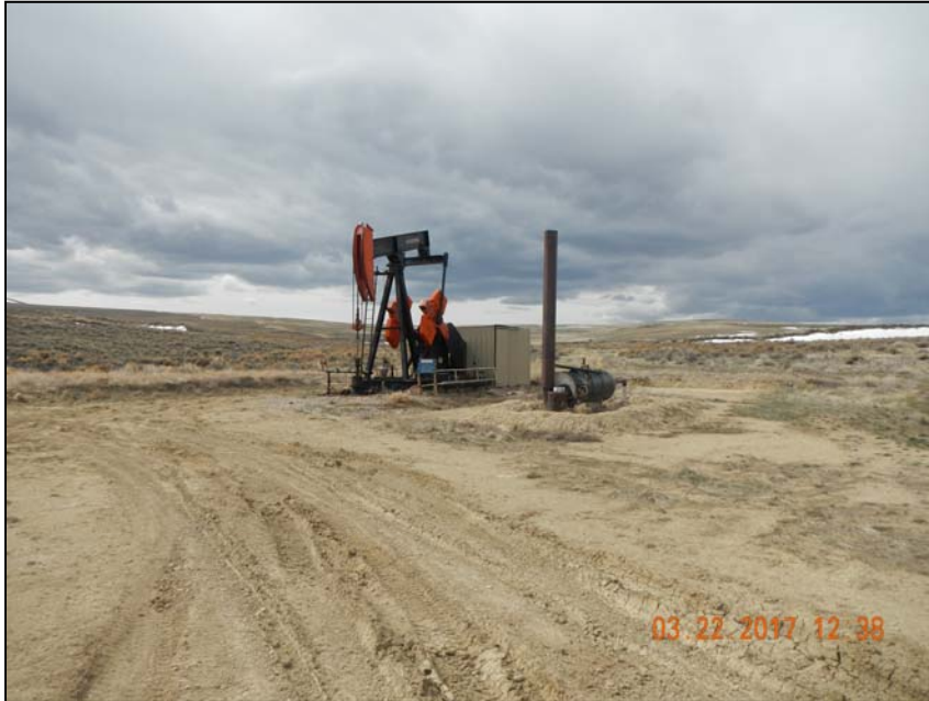
Photo 2. ~18 foot setback between pump jack and heated separator.
