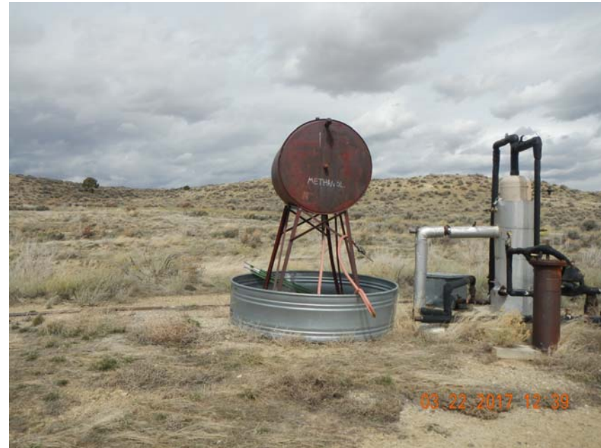
Photo 4. Partially labeled methanol container.
