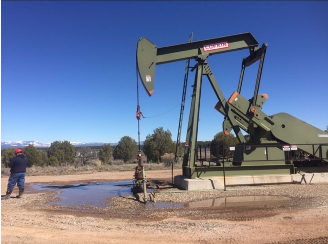
Figure 1. A well head packing leaked causing 2 bbl of CBM produced water to be released onto the location around the well head. This photograph was taken looking north east.
