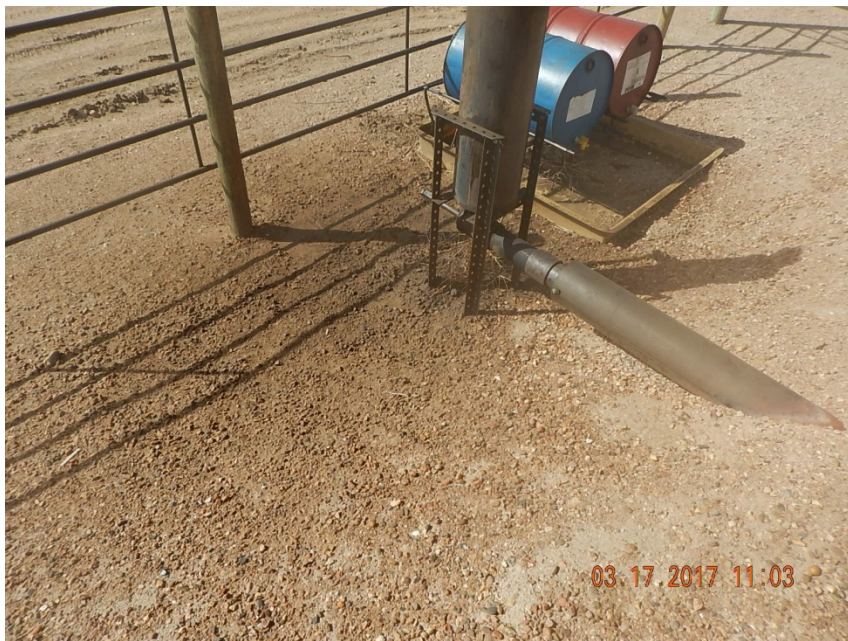
Photo 1: Stained soil at exhaust
