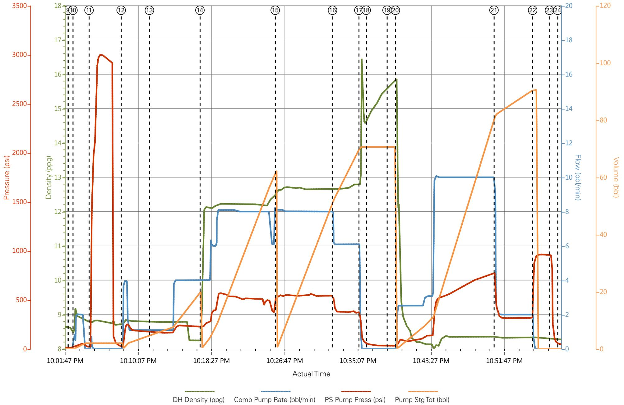
⑨ Start Job ⑩ Prime Pumps ⑪ Test Lines ⑫ Pump Spacer 1 ⑬ Check weight ⑭ Pump Lead Cement ⑮ Pump Tail Cement ⑯ Slow Rate ⑰ Shutdown ⑱ Drop Top Plug ⑲ Wash On Top
