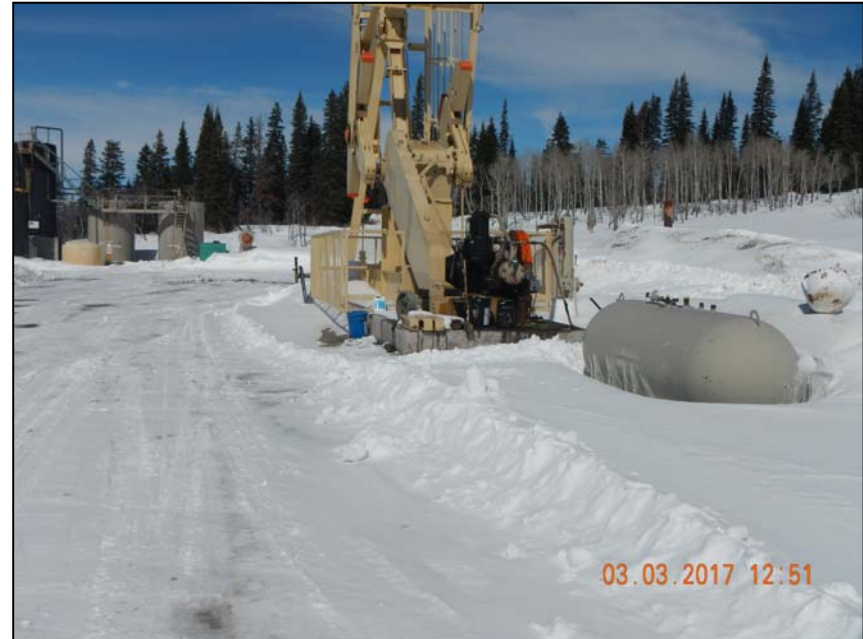
Photo 7. Lube oil containers stored on pump jack base with no containment.
