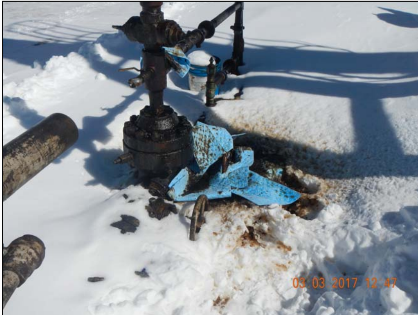
Photo 6. Absorbent pads with lube oil container with no containment in background.
