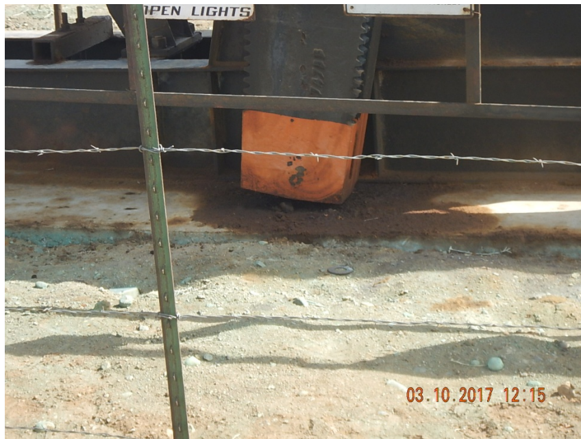
Photo 4: Stained soil at pump jack
