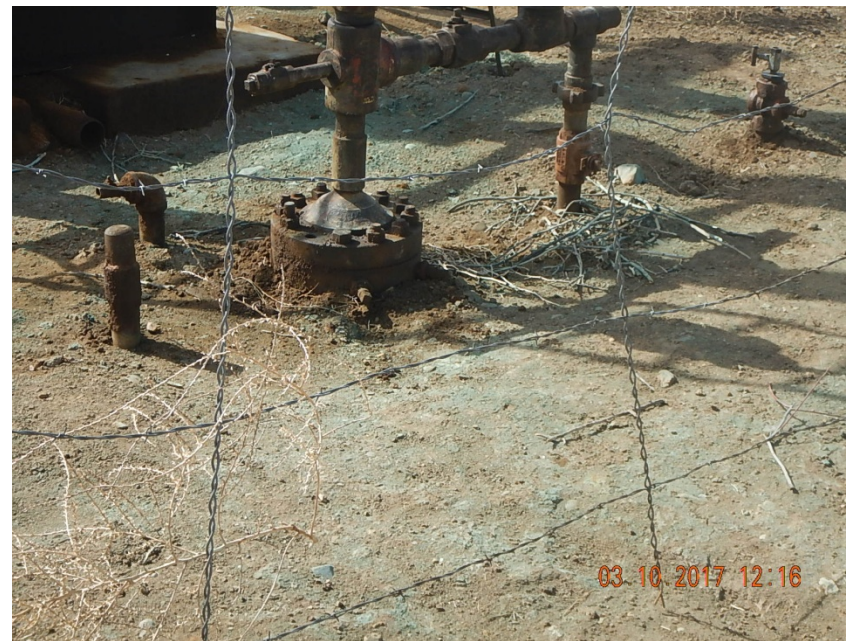
Photo 5: Stained soil at wellhead
