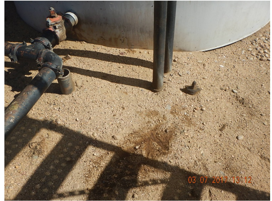
Photo 2: Stained soil at tank loadout
