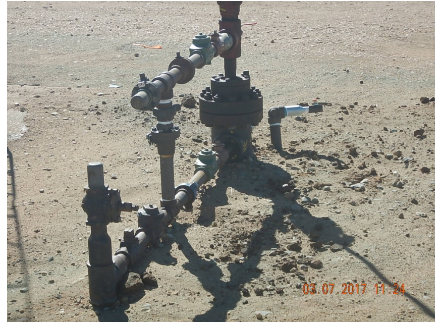
Photo 1: Bradenhead plumbed to surface
