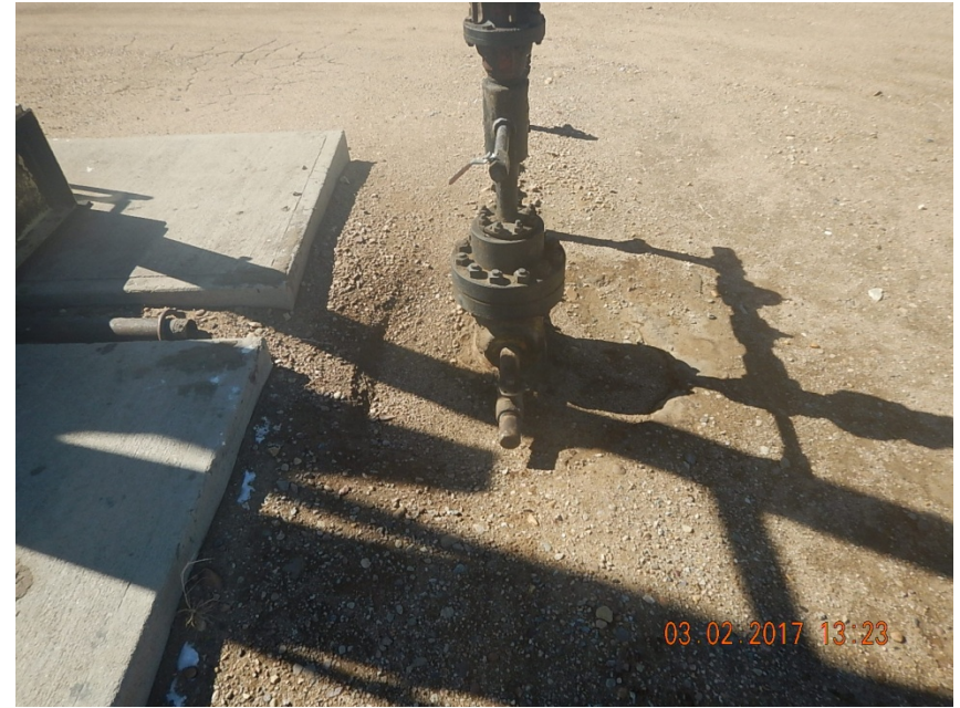
Photo 4: No bradenhead at surface
