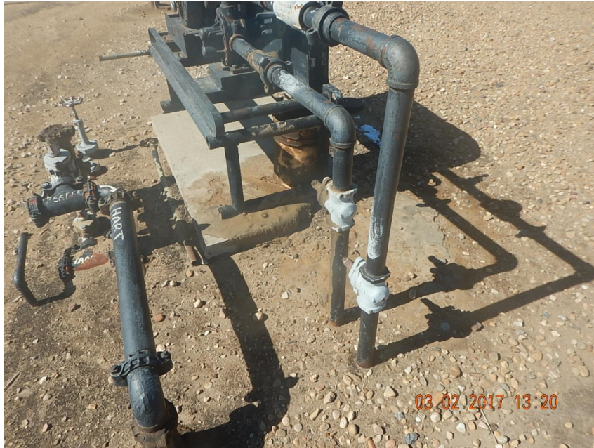
Photo 1: Stained soil at small engine
