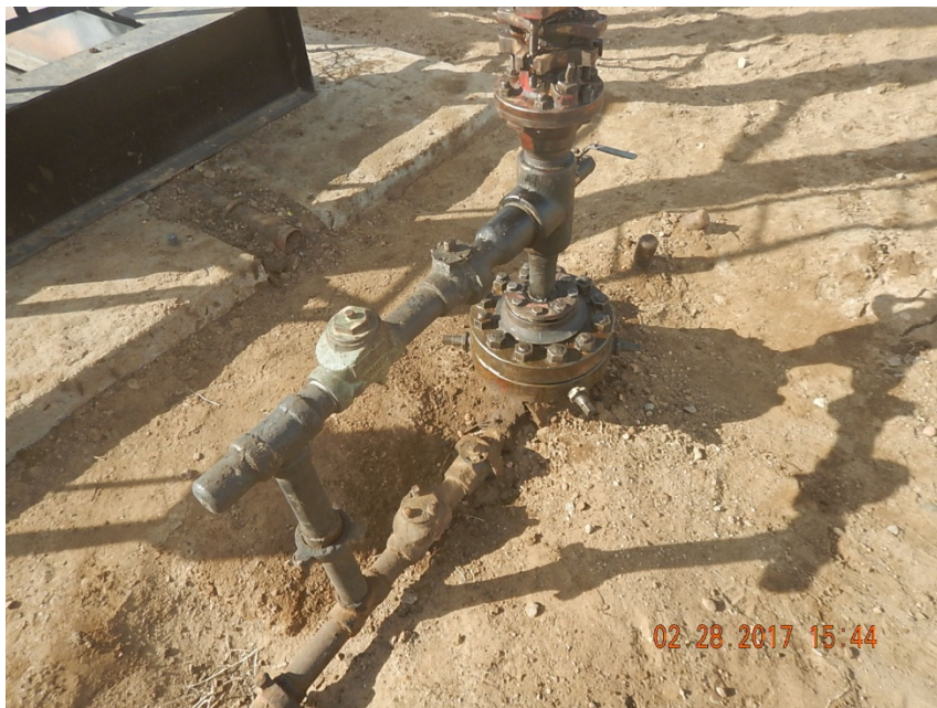
Photo 2: Stained soil at wellhead, no bradenhead plumbed to surface.
