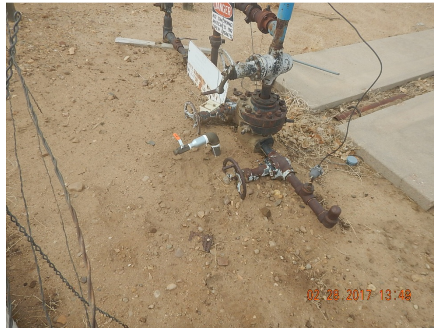
Photo 1: Bradenhead at surface, stained soil at wellhead removed.
