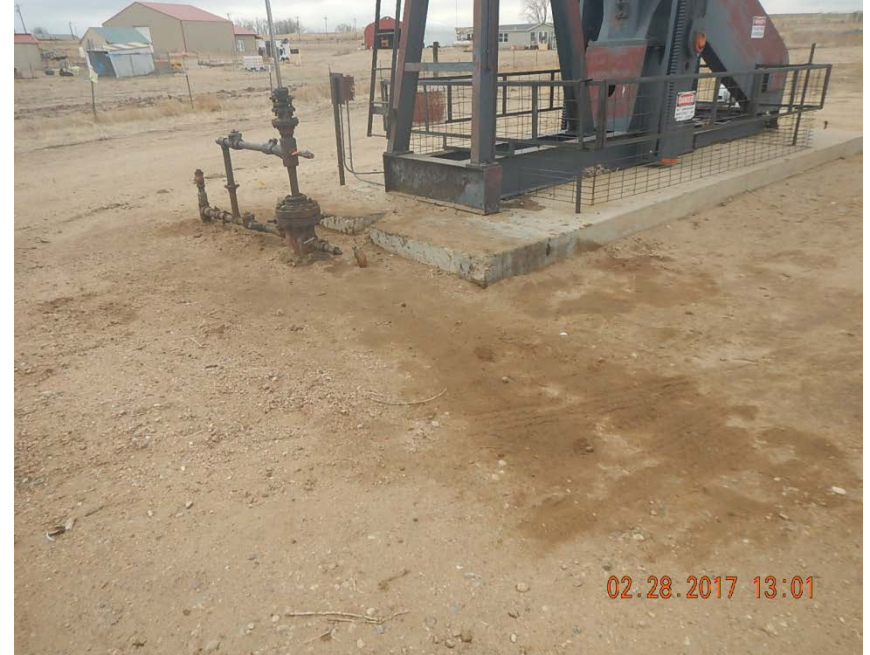
Photo 1: Stained soil at wellhead, looking SW
