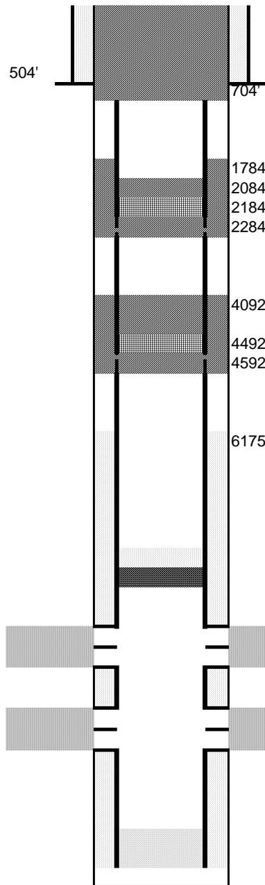
Cut surface casing off 6'-8' below surface.
