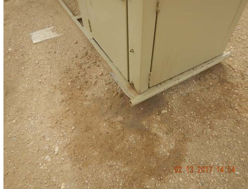
Photo 7: Stained soil at NW corner of separator
