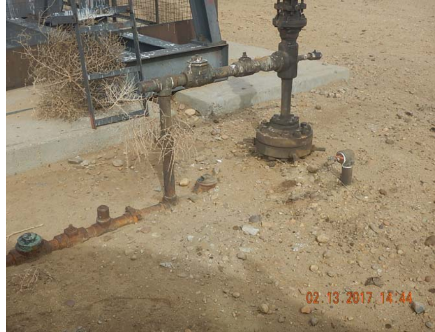
Photo 1: Stained soil removed at wellhead
