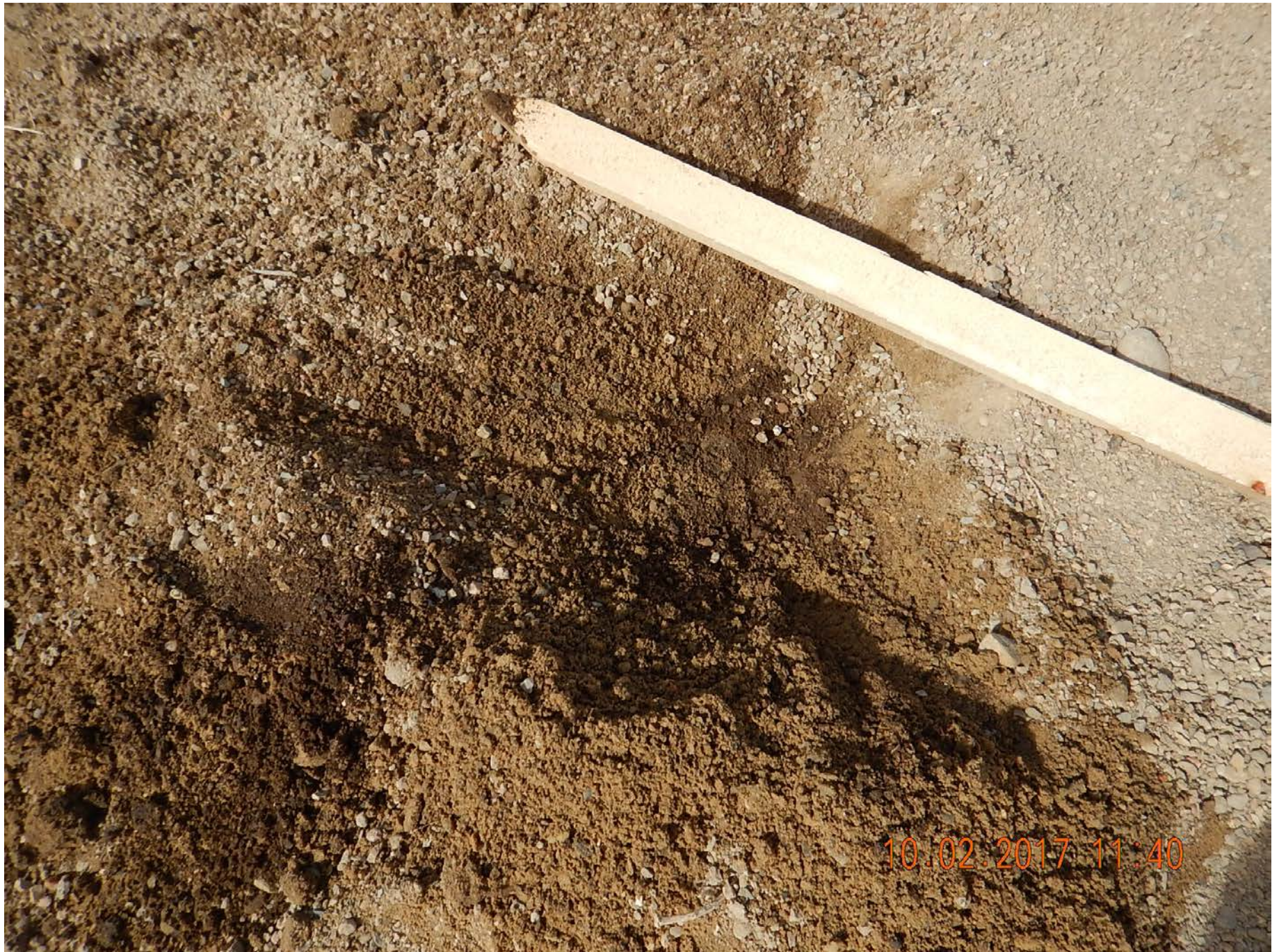
A small excavation adjacent to wellhead found stained soil with a strong hydrocarbon odor.
