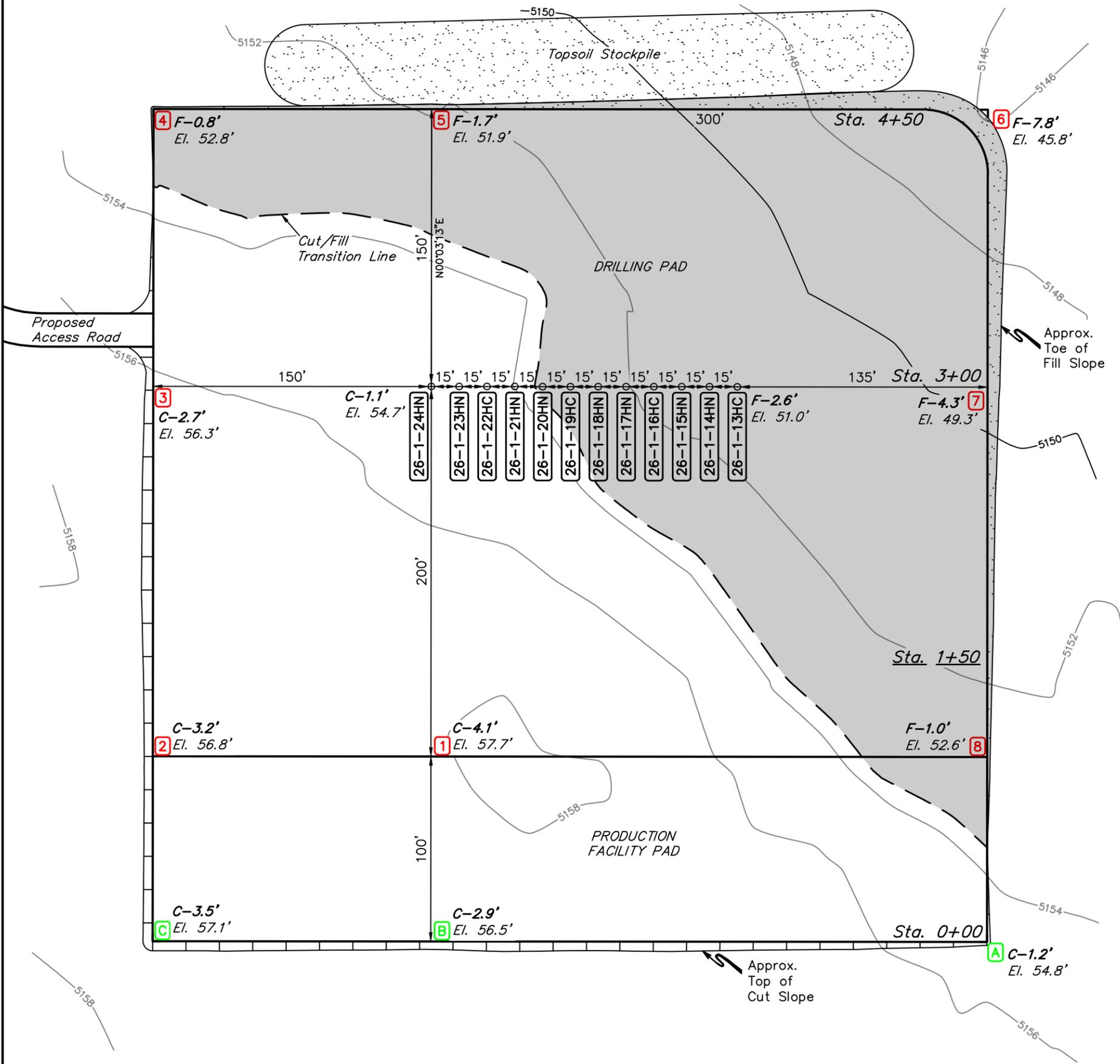
NOTE: Earthwork calculations require a fill @ some location stakes for balance. All fill is to be compacted to a minimum of 95% of the maximum dry density obtained by AASHTO method t-99.
