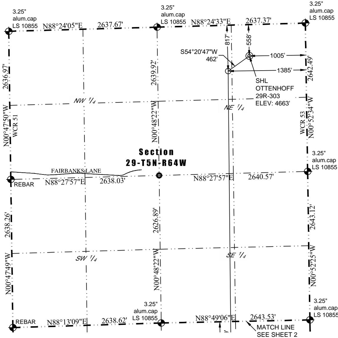
In accordance with a request from Paul Montville of PDC Energy, Inc., Washburn Land Surveying, LLC has determined the location of the **OTTENHOFF 29R-303** well site to be SHL: 558' FNL and 1005' FEL, (BHL: 2340' FNL and 1433' FEL), as measured at ninety (90) degrees from the section lines of Sections 29 and 32, Township 5 North, Range 64 West of the 6th Principal Meridian, Weld County Colorado.
