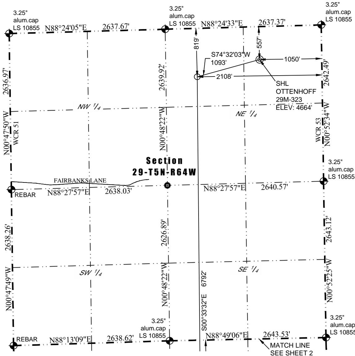
In accordance with a request from Paul Montville of PDC Energy, Inc., Washburn Land Surveying, LLC has determined the location of the **OTTENHOFF 29M-323** well site to be SHL: 557' FNL and 1050' FEL, (BHL: 2340' FNL and 2157' FEL), as measured at ninety (90) degrees from the section lines of Sections 29 and 32, Township 5 North, Range 64 West of the 6th Principal Meridian, Weld County Colorado.
