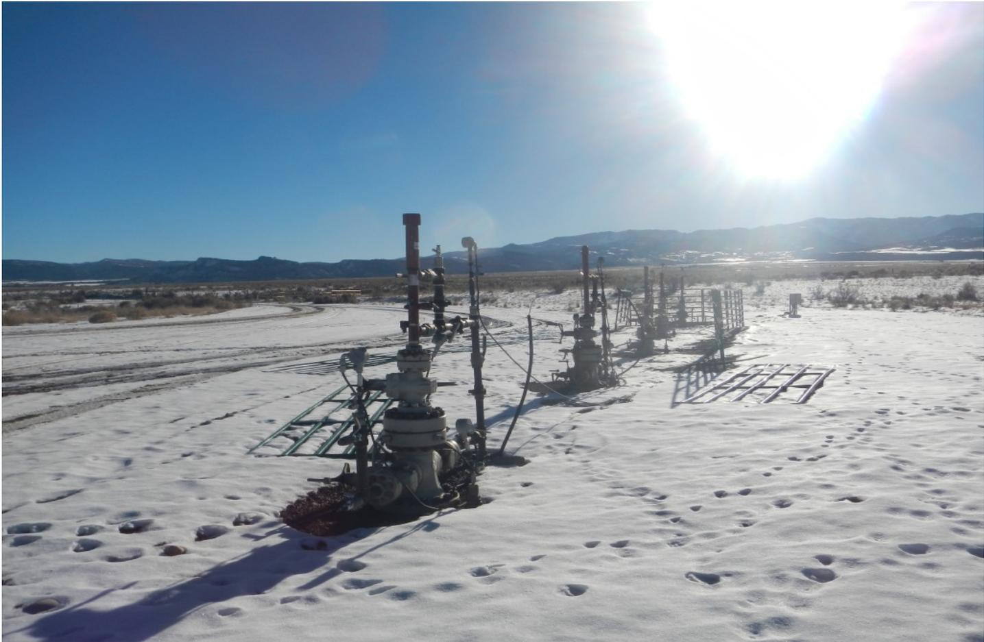
Photo#2: There is no evidence of the AL Well on this Active Location with Five PR Wells
