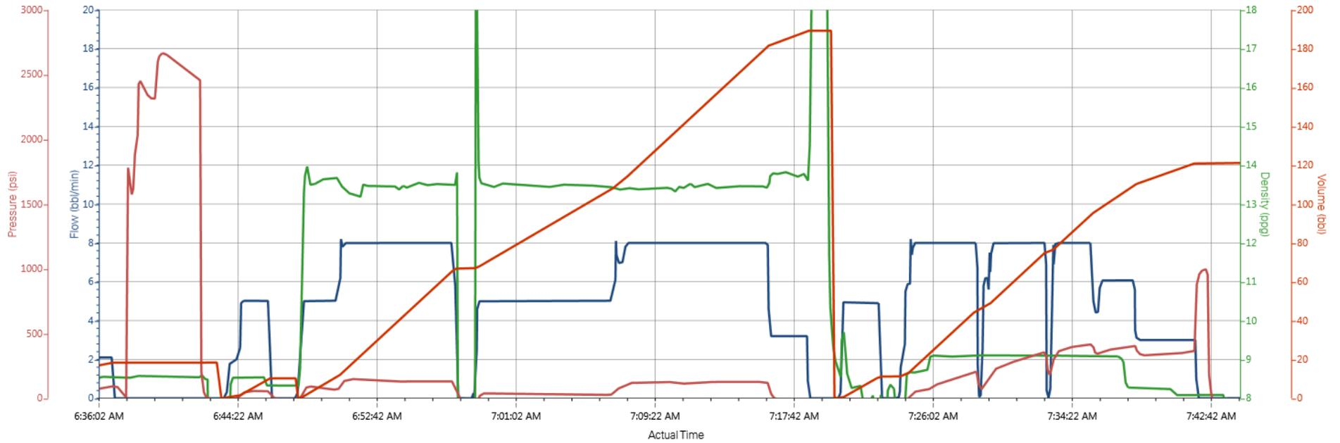
Comb Pump Rate (bb/min) DH Density (ppg) PS Pump Press (psi) Pump Stg Tot (bbl)
