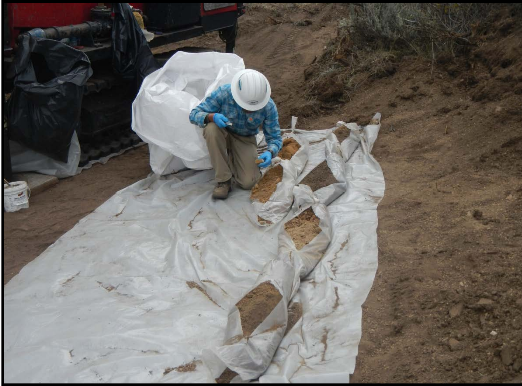
Geologist analyzing core samples. Mostly fine poorly cemented sandstone observed on MWs drilled on the west and east flanks of the valley. Rotasonic vibration pulverizes poorly cemented sandstone. Looks like sand...
