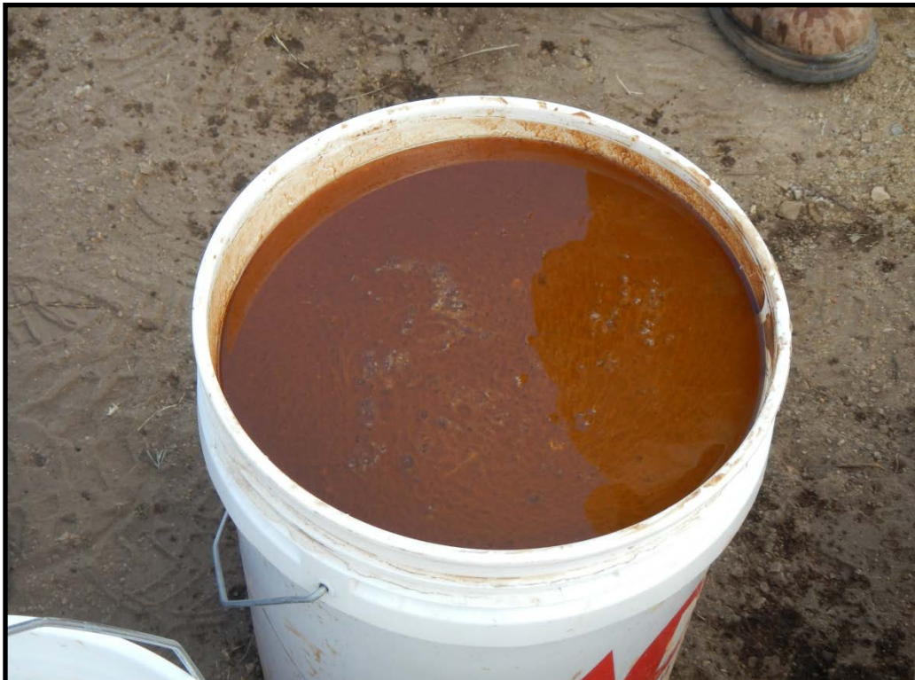
Free product has an orange color. Compare color with clay on last slide of this presentation.
