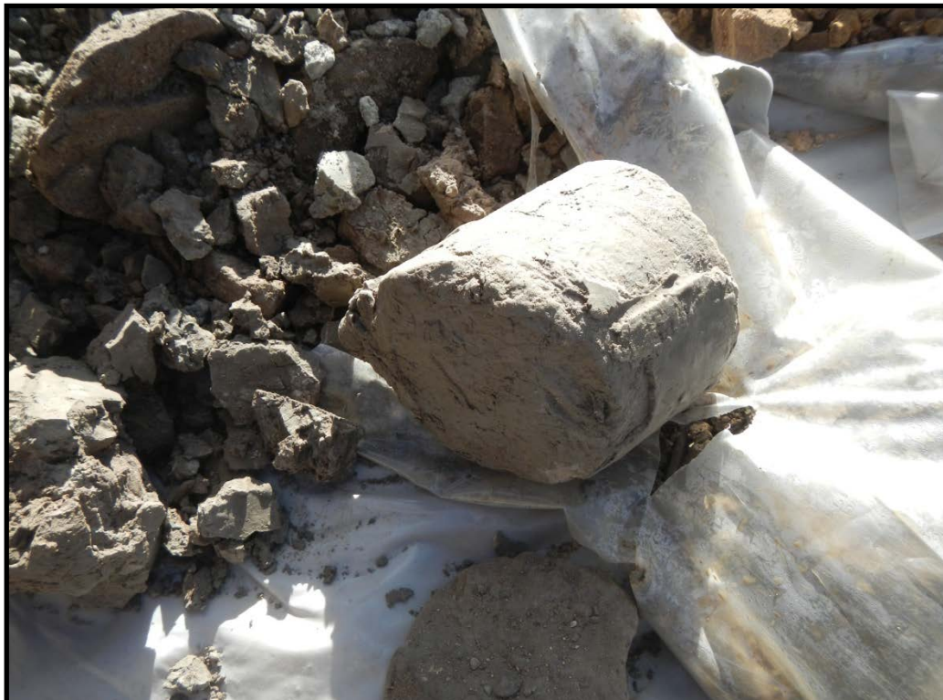
Bedrock of hard sandstone on MW-19 (west side of the gulch). Depending on location and elevation, well depth between 50 and 70 feet, typically about 10 to 20 feet of water in well.
