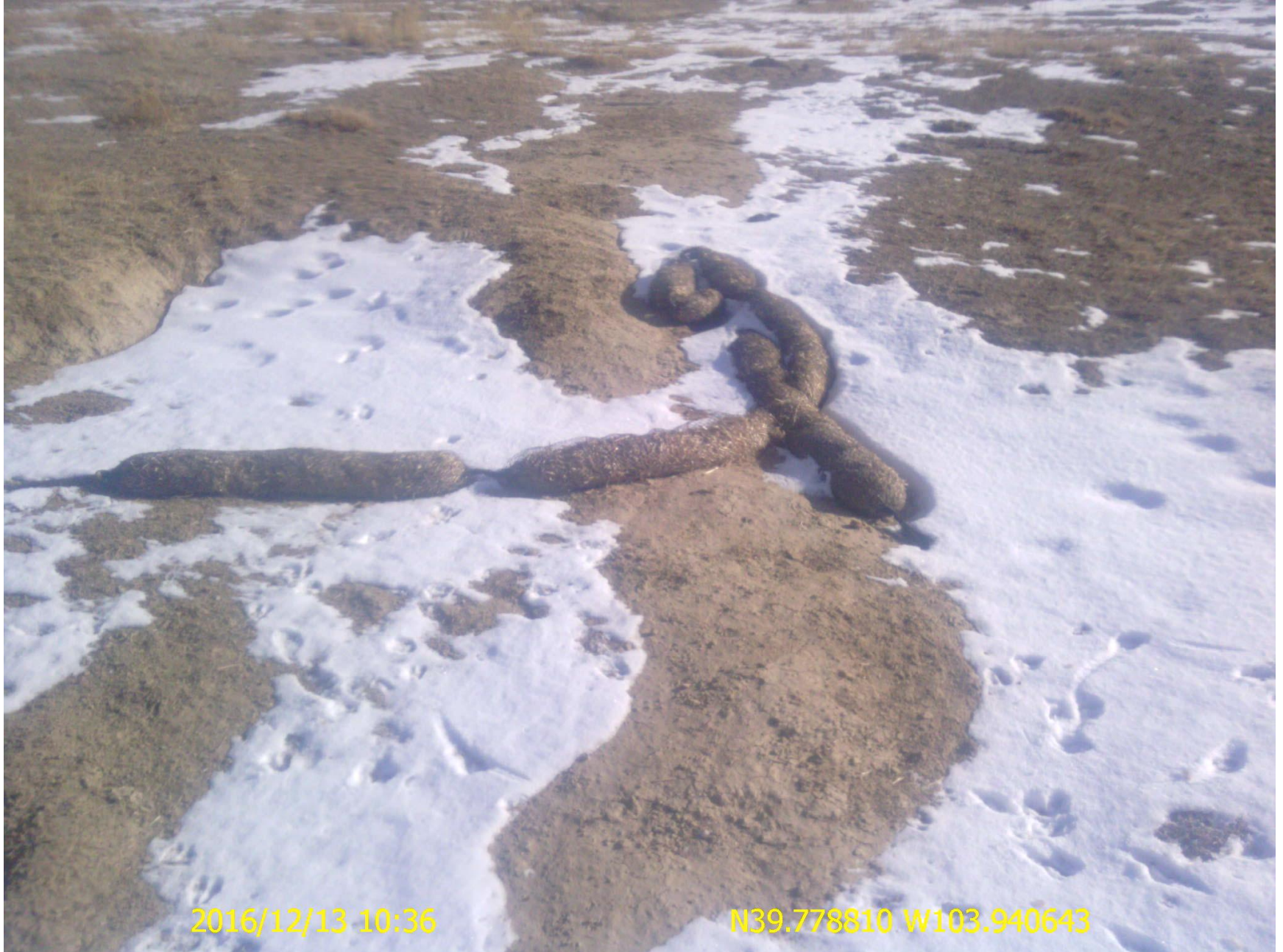
Figure 7: Photo taken from the northern disturbance area, facing east towards the access road. Photo shows erosion has not been stabilized or reclaimed. Refer to photos from inspection Doc. # 682500938 for additional details.
