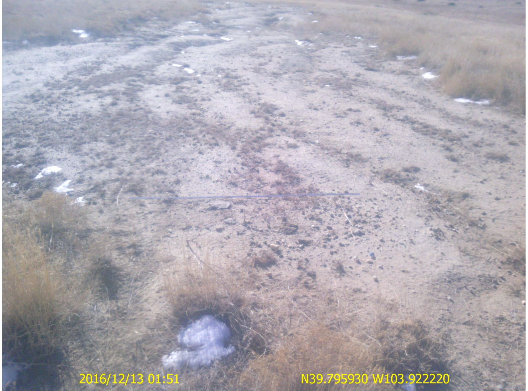
Figure 3: Photo taken from the south end of the location, facing south. Photo shows large un-vegetated area experiencing erosion. Photo shows stormwater and sediment control BMPs have not been installed. See photos from inspection Doc. #682501125 for additional information and details
