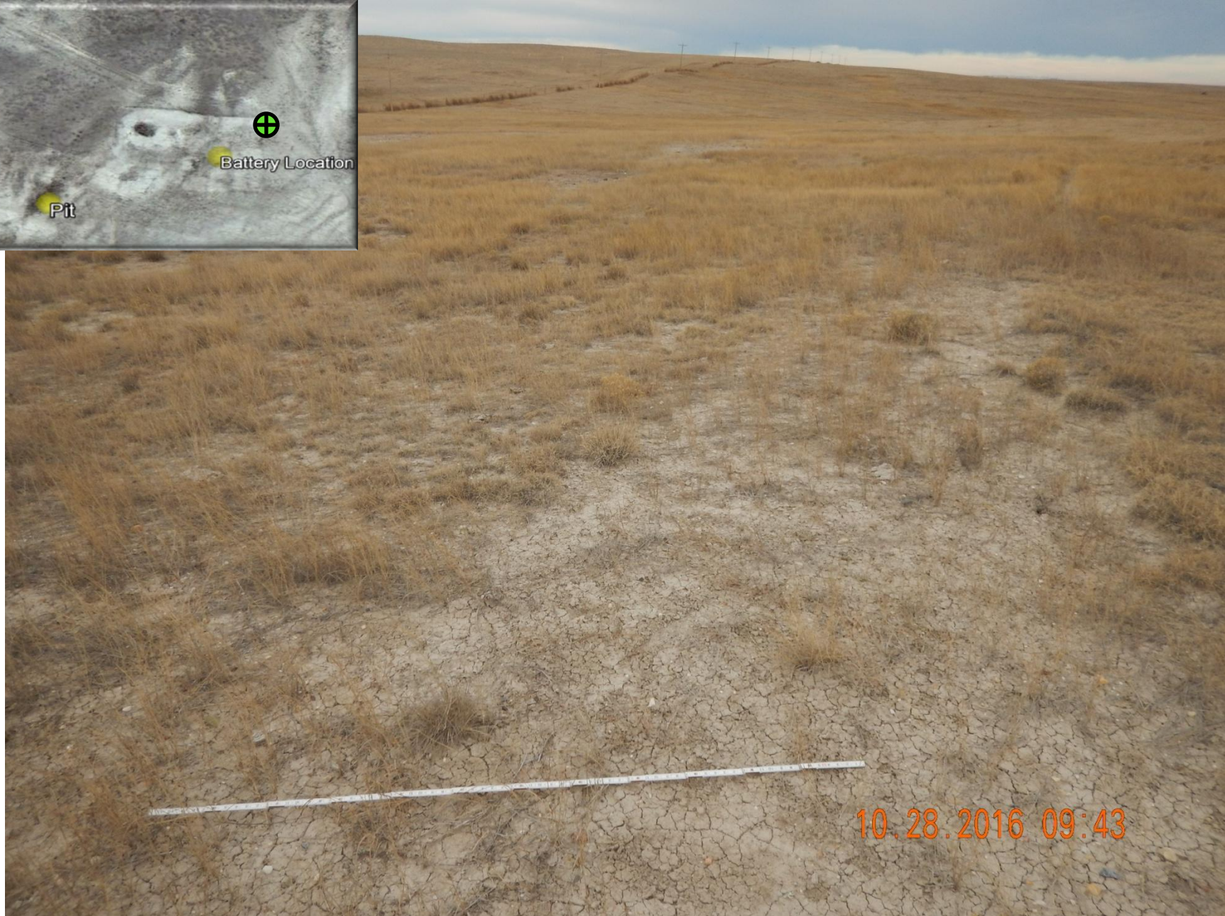
Figure 34: Photo taken from the northeast corner of the battery location, facing west. Photo shows areas pit/battery location has not achieved uniform vegetative cover and large areas remain unvegetated. 6' measuring stick for reference.
