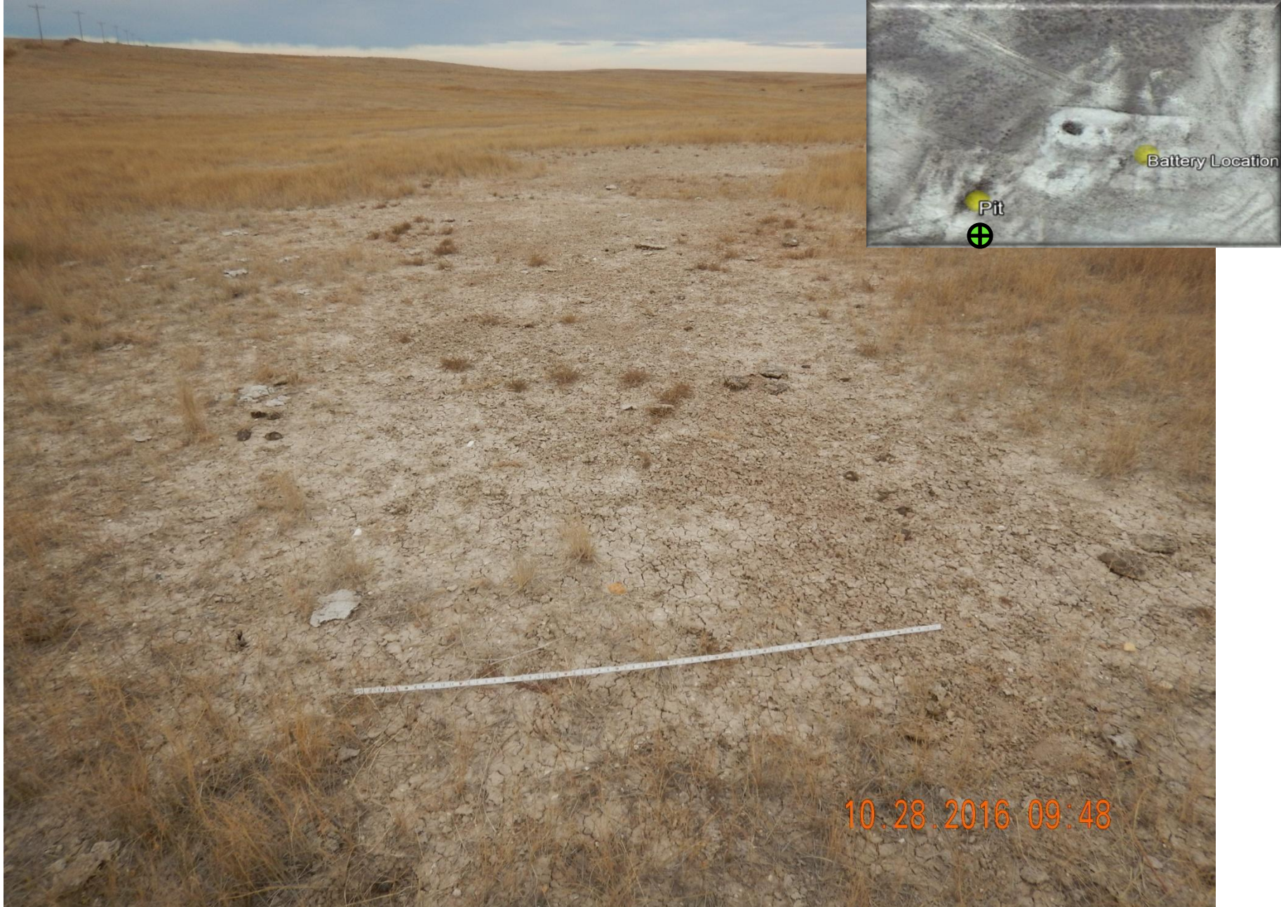
Figure 48: Photo taken from southeast end of the pit location, facing west. Photo shows areas pit/battery location has not achieved uniform vegetative cover and large areas remain unvegetated. 6' measuring stick for reference.
