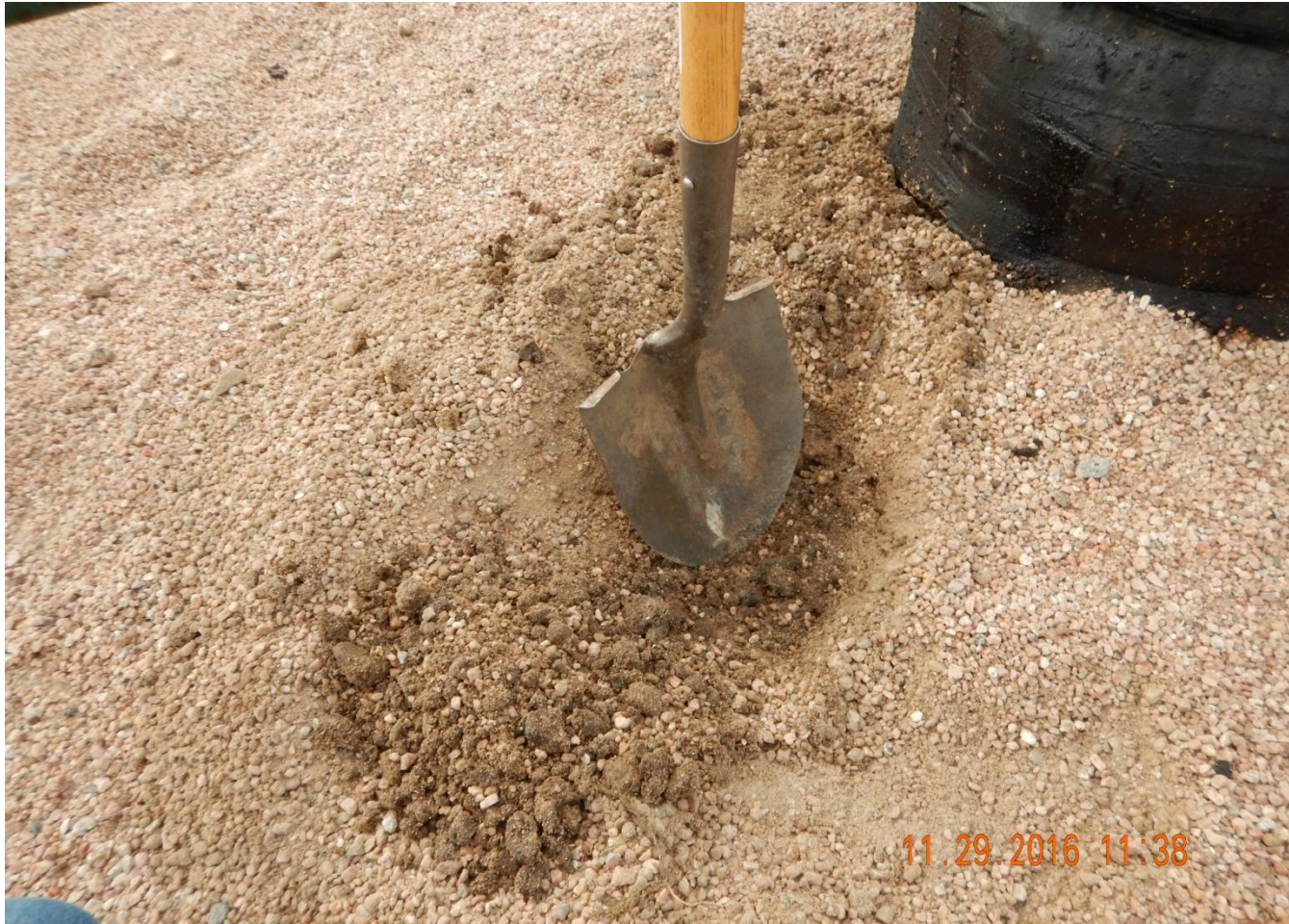
Photo 5. Photo taken at wellhead. It appears the impacted soil around the wellhead has not been removed. Removal of 3"-4" of gravel on top reveals stained soil with a hydrocarbon like odor.
