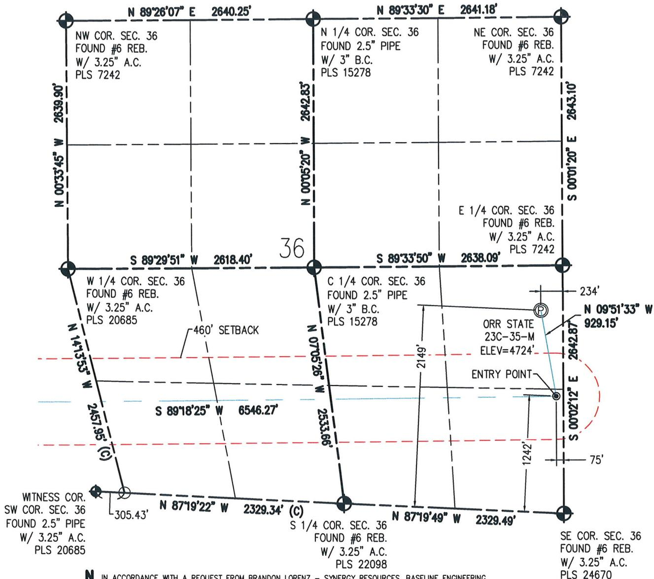
**N** IN ACCORDANCE WITH A REQUEST FROM BRANDON LORENZ - SYNERGY RESOURCES, BASELINE ENGINEERING CORP. HAS DETERMINED THE LOCATION OF THE ORR STATE 23C-35-M TO BE 2149' FSL AND 234' FEL, AS MEASURED AT NINETY (90) DEGREES FROM THE SECTION LINE OF SECTION 36, TOWNSHIP 6 NORTH, RANGE 67 WEST AND THE BOTTOM HOLE LOCATION TO BE 858' FSL AND 1674' FEL OF SECTION 35, TOWNSHIP 6 NORTH, RANGE 67 WEST, 6TH PRINCIPAL MERIDIAN, WELD COUNTY, COLORADO.
