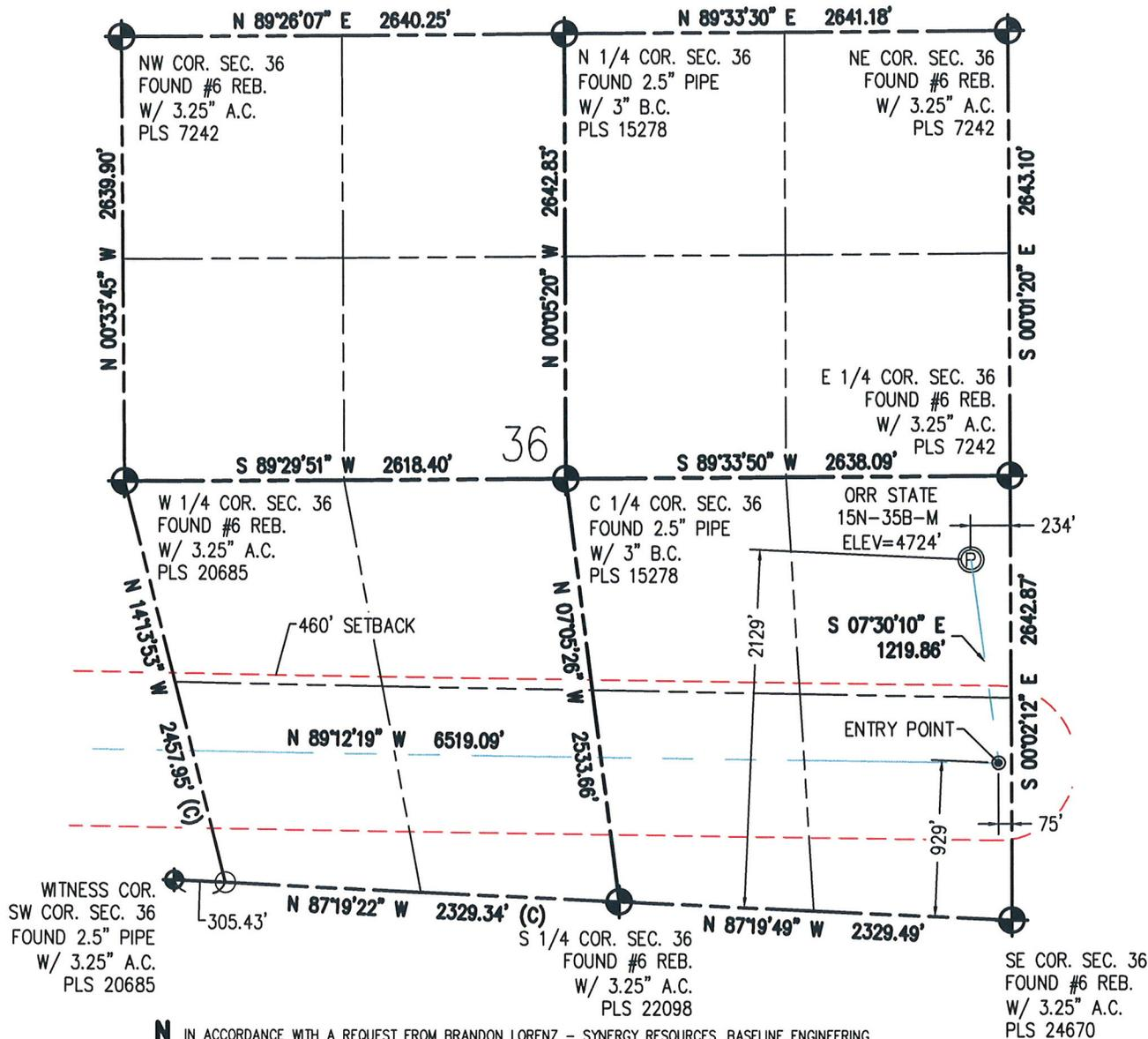
**N** IN ACCORDANCE WITH A REQUEST FROM BRANDON LORENZ - SYNERGY RESOURCES, BASELINE ENGINEERING CORP. HAS DETERMINED THE LOCATION OF THE ORR STATE 15N-35B-M TO BE 2129' FSL AND 234' FEL, AS MEASURED AT NINETY (90) DEGREES FROM THE SECTION LINE OF SECTION 36, TOWNSHIP 6 NORTH, RANGE 67 WEST AND THE BOTTOM HOLE LOCATION TO BE 715' FSL AND 1683' FEL OF SECTION 35, TOWNSHIP 6 NORTH, RANGE 67 WEST, 6TH PRINCIPAL MERIDIAN, WELD COUNTY, COLORADO.
