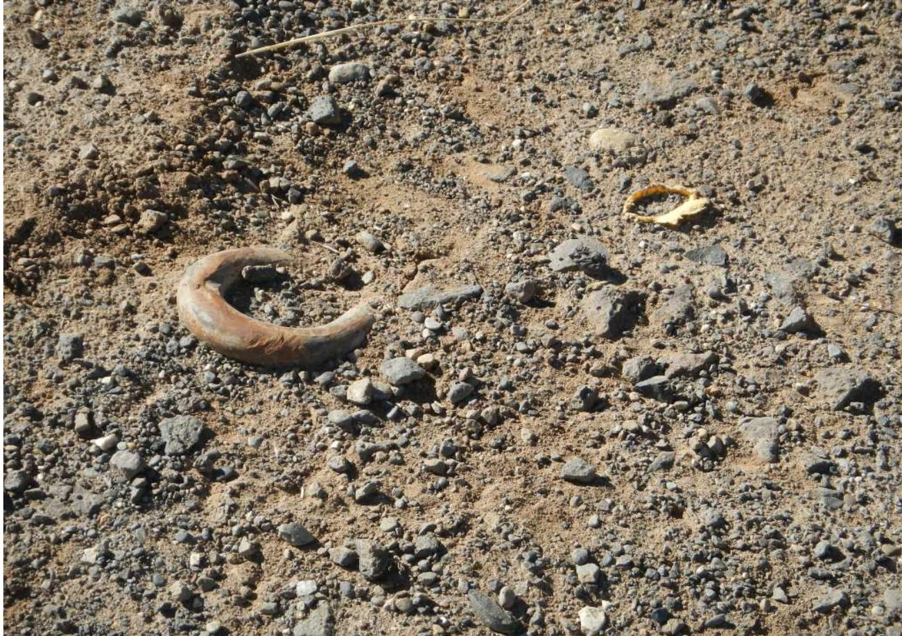
Photo#4: Guy Anchor; smashed and Marker broken off.
