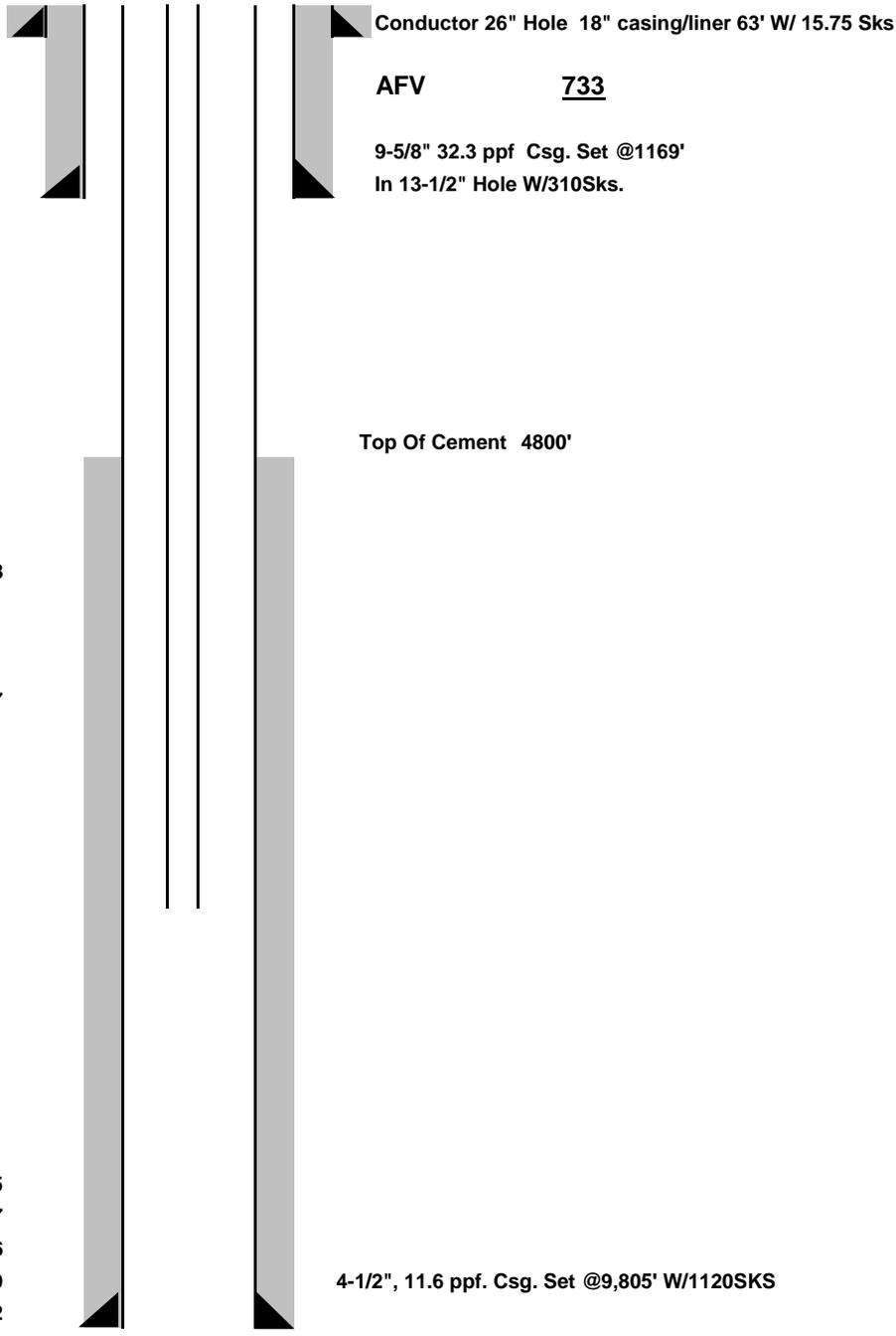
Conductor 26" Hole 18" casing/liner 63' W/ 15.75 Sks
