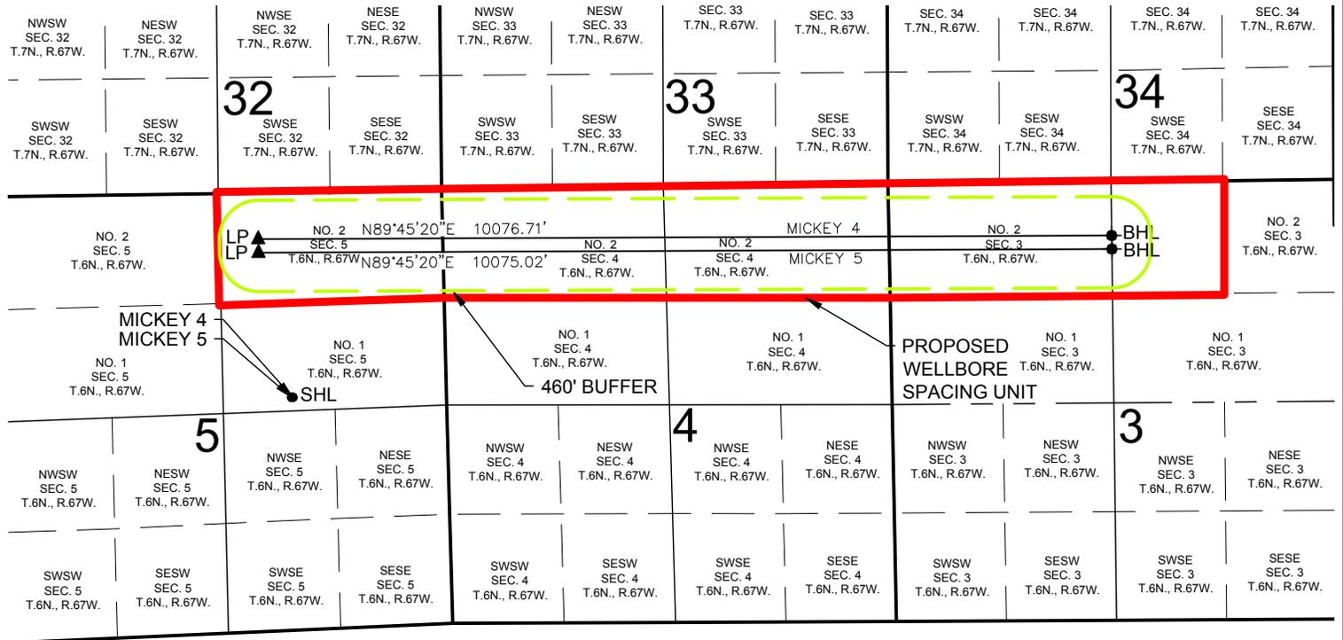
**WELL MICKEY 4 TO BE LOCATED 2419' FNL AND 1813' FEL, SEC. 5, T6N, R67W
