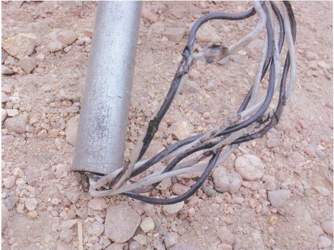
8. Meter's electrical wires show minor melting of insulation and mechanical damage, but no arcing.
