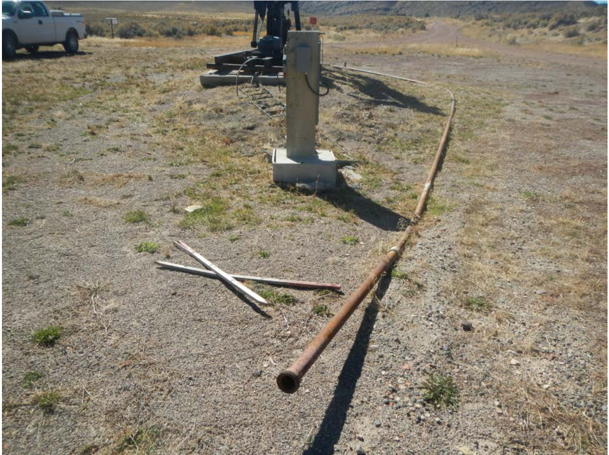
Flowline from wellhead
