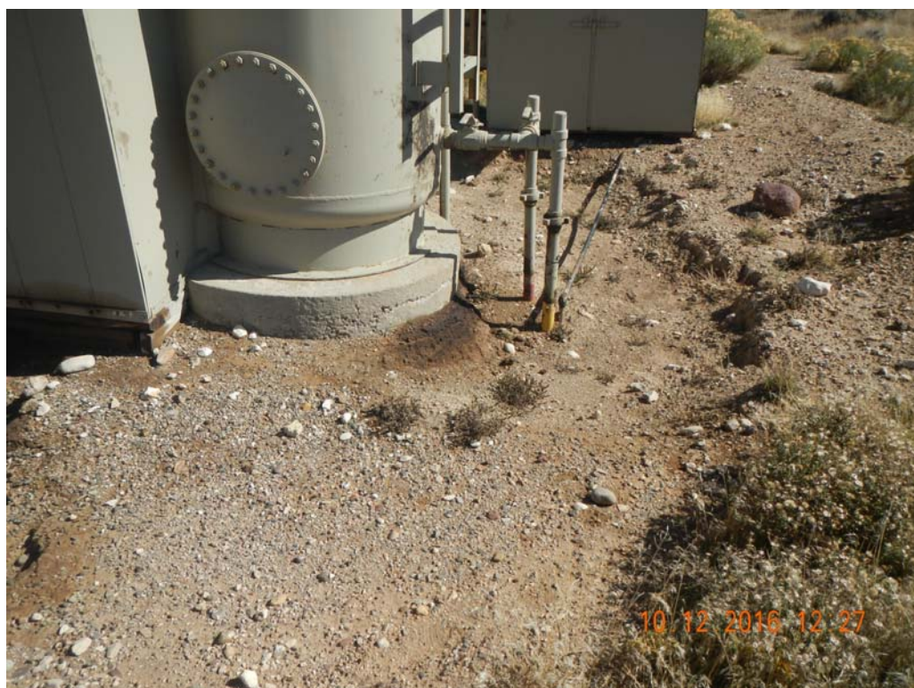
Stained soil and dugout area from apparent spill.
